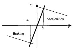
Fig. 4. Approximation of slip characteristic curve.
