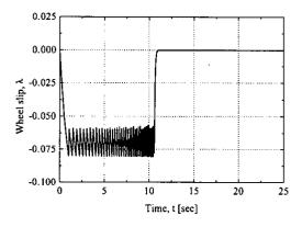
Fig. 10. Wheel slip trajectory.
