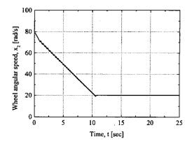
Fig. 9. Wheel angular speed trajectory.
