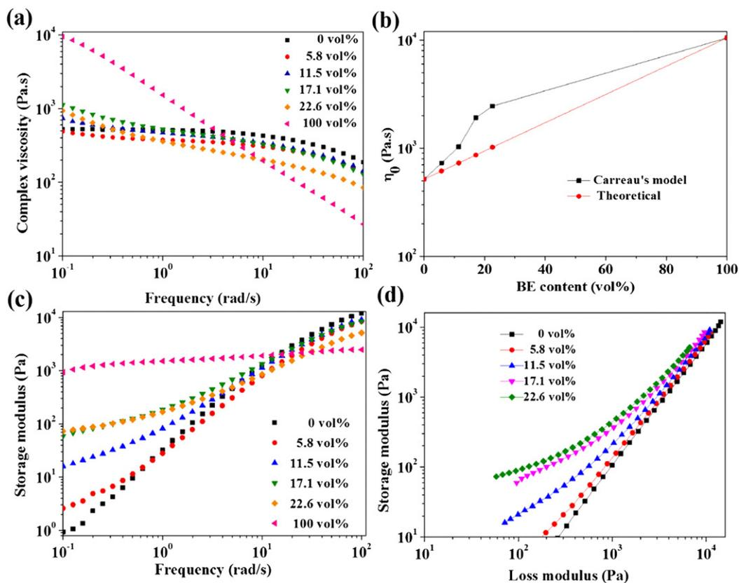
**Fig. 6.** Rheological properties of PLA/BE blends with different amounts of BE: (a) complex viscosity ( $\eta$ ); (b) Newtonian viscosities ( $\eta_0$ ) vs compositions; (c) storage modulus ( $G'$ ); (d) storage modulus vs loss modulus.
