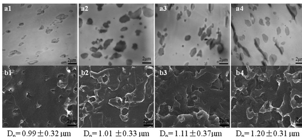
Fig. 2. Micrographs of PLA/BE blends with (a1, b1) 5.8 vol% BE, (a2, b2) 11.5 vol% BE, (a3, b3) 17.1 vol% BE, and (a4, b4) 22.6 vol% BE. a: TEM micrographs; b: SEM micrographs;  $D_n$ : The number-average particle diameter.
