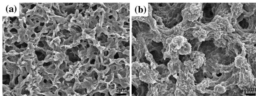
Fig. 9. SEM micrographs of etched samples: (a) PLA; (b) PLA/BE blend (11.5 vol% BE).
