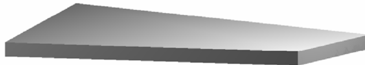
Figure 8. Warped precast slabs.
