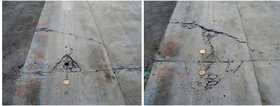
Figure 16. End of life at the two joints of section 1, loaded to failure.
