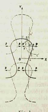
Fig. 1 Forces acting in the plain-knit structure Equilibrium of the loop segments
