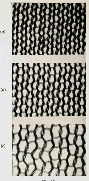
Fig. 13 Dry-relaxed silk fabrics (a) sample 1 (K = 16.1) (b) sample 3 (K = 14.0) (c) sample 6 (K = 10.0)
