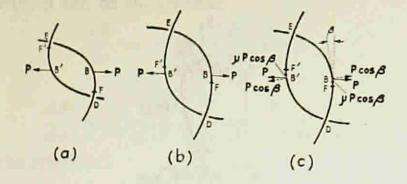
Fig. 5 Diagram showing the forces acting on the loop (a) in a distorted condition (b) in the relaxed condition (c) in the relaxed condition, showing the elastic and frictional components
