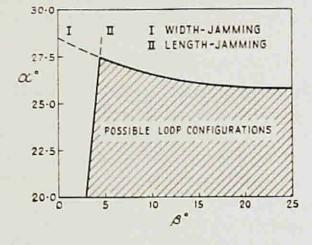
Fig. 8 Relation between  $\alpha$  and  $\beta$  for the jamming conditions
