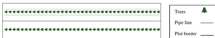
Fig. 1. A schematic plan of the experimental units (surface irrigation plot as well as subsurface irrigation plot showing the position of pipe lines)
