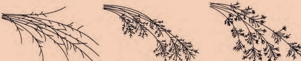
(a) Sparks from 1015 steel (0.15% C). (b) Sparks from 1045 steel (0.45% C). (c) Sparks from 1095 steel (1.0% C)
