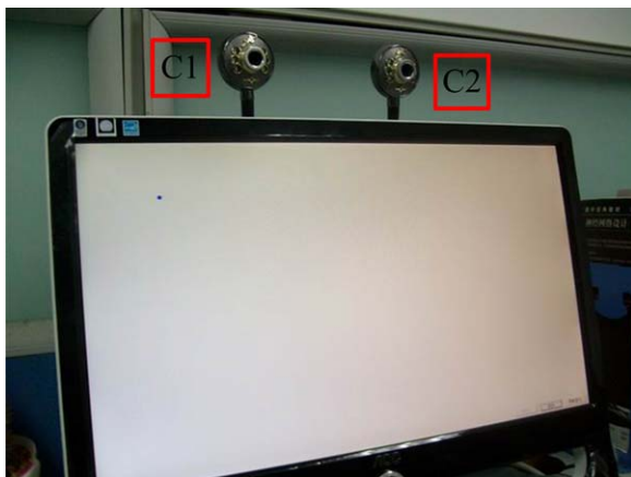
Fig. 6. Cameras C_1 , C_2 are used to measure the spatial coordinates of the observer's eyes; the image captured by C_2 is also used to compute the LPM features. The screen dimensions are 1024 \times 786 .
