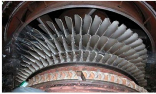
Fig. 19. Fracture of the first four stage blades [106].
