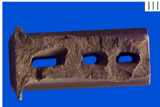
Fig. 14. Upper view of the fracture surface of the blade that was identified as the origin of the failure [90].
