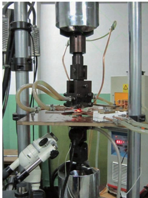
Fig. 20. Thermo-mechanical fatigue test system for blades [164].
