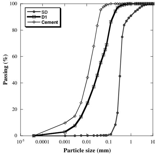
Fig. 2. Size distributions of the various granular elements added into the mixes.
