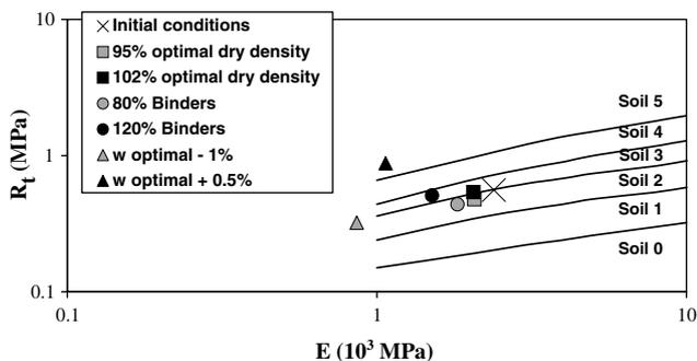
Fig. 9. Influence of the variability of dry density, binder proportion and water content on the mechanical behaviour of mix 2.
