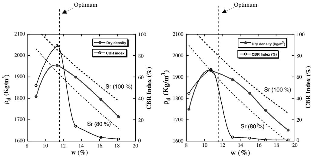
Fig. 5. Level of compaction and bearing of mix 1 (left) and mix 2 (right).
