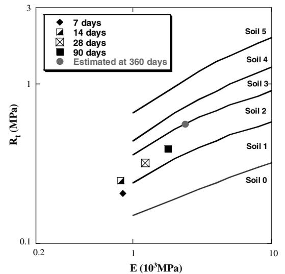
Fig. 7. Evolution of the mechanical behaviour of the mix 2 with time.
