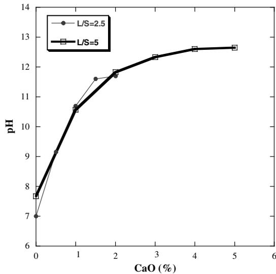
Fig. 3. Evolution of the pH for a sediment solution according to the lime addition.
