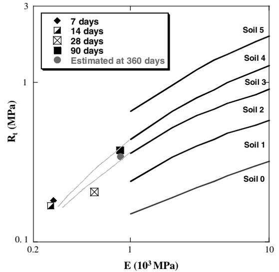
Fig. 6. Evolution of the mechanical behaviour of the mix 1 with time.
