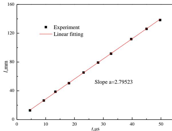
**Figure 3.** Linear fitting curve of the experimental results, the slope represents the velocity of surface wave propagation in the TC4 base material.
