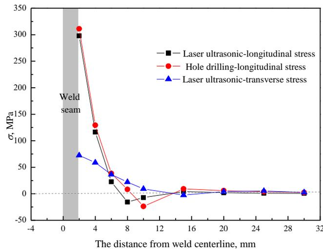
**Figure 6.** The residual stress distribution in TC4 laser welding at a welding power of 2800 W, welding speed of 6.0 m/min, and heat input of 28 kJ/m. The longitudinal residual stresses measured by the hole-drilling method and ultrasonic laser method were consistent.
