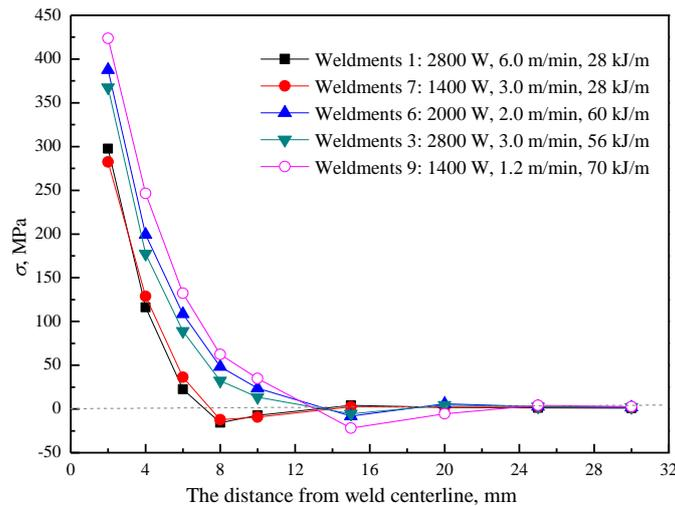
**Figure 8.** Longitudinal residual stress distribution with different heat inputs.
