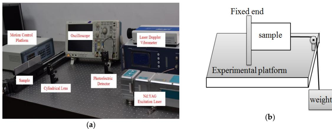
**Figure 1.** Experimental system: (a) ultrasonic laser and (b) pre-stress loading apparatus.
