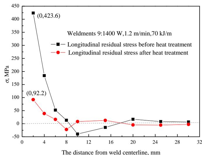
**Figure 11.** Comparison of the longitudinal residual stress before and after heat treatment. The maximum of longitudinal residual stress was reduced from 423 MPa to 92 MPa, a decrease of 78%.
