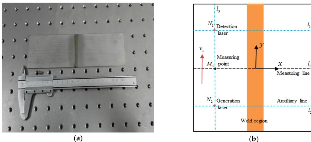
**Figure 5.** (a) Experimental specimen and (b) layout of measuring line when measuring the velocity  $v_y$ , where  $M_0$  is a measurement point;  $l_0$  is the measuring line;  $l_1$ ,  $l_2$ , and  $l_3$  are the auxiliary lines; and  $N_1$  and  $N_2$  are the positions of the laser beam.
