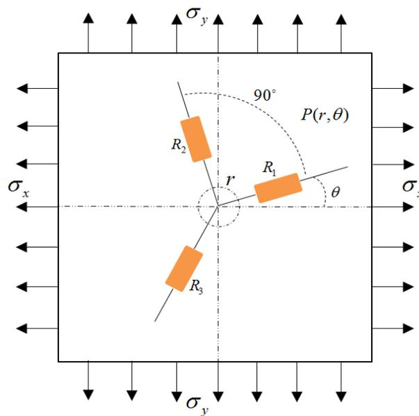
**Figure 7.** Diagram of sensitive grid arrangement  $\theta$  is the angle between the principal stress  $\sigma_x$  and the strain gauge  $R_1$ , and the angle between the strain gauge  $R_2$  and  $R_3$  is  $135^\circ$ .
