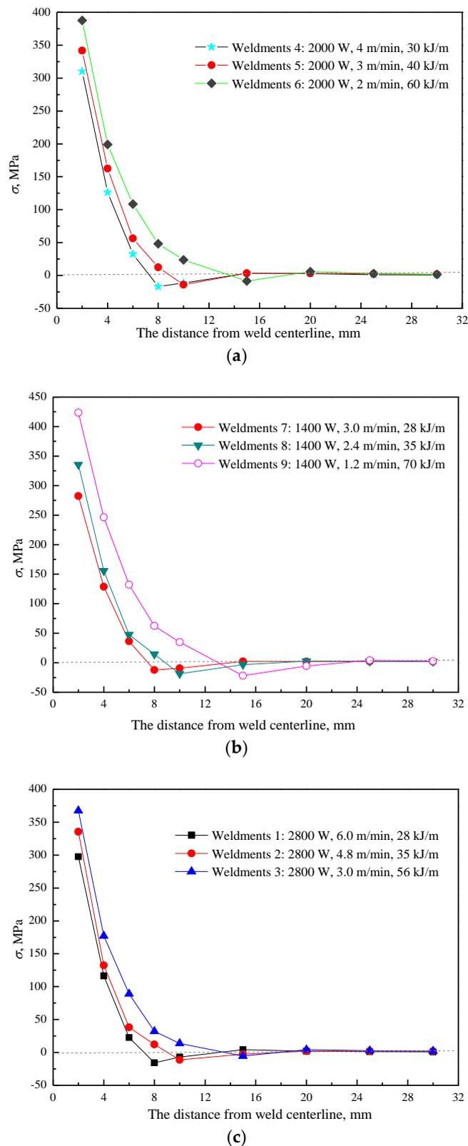
**Figure 10.** The longitudinal residual stress distribution with the same welding power: (a) 2000 W, (b) 1400 W, and (c) 2800 W.
