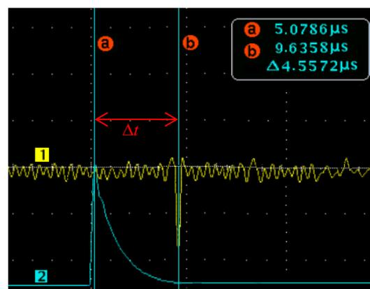
**Figure 2.** Travel time of surface waves in the base material without stress. The change in distance is  $\Delta l = 12.82$  mm, Channel 1 is the vibration signal, Channel 2 is the time reference signal, a and b are the cursors for reading travel time.
