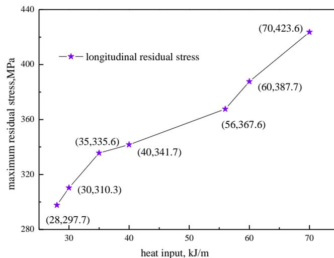
**Figure 9.** The relationship between maximum longitudinal residual stress and heat input. Three approximate linear stages are presented and the maximum residual stress changes slowly in the second stage.
