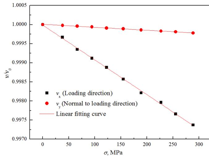
**Figure 4.** The relationship between velocity ratio and tensile stress. The slopes of the linear fitting curve correspond to the acoustoelastic coefficients.
