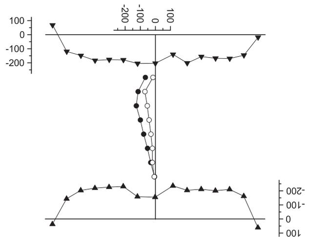
Fig. 6. Residual stress distribution in R-H-3 by sectioning method.
