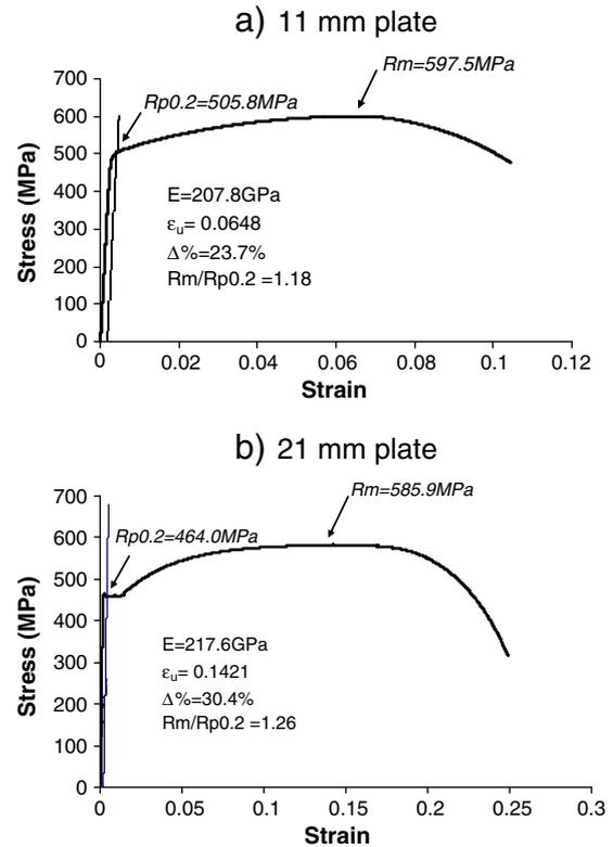
Fig. 1. Stress–strain curve for Q460 steel.
