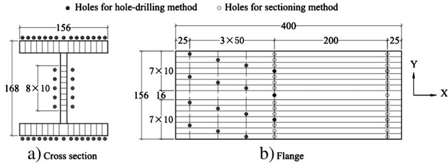
Fig. 4. Distribution of hole drilling and sectioning for R-H-3.
