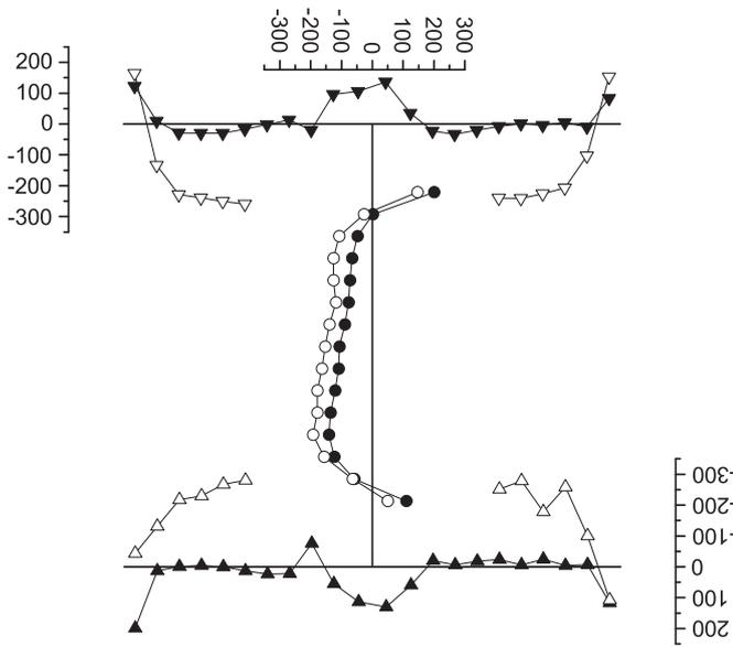
Fig. 7. Residual stress distribution in R-H-5 by sectioning method.
