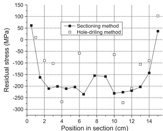
Fig. 10. Comparison of the hole-drilling method and the sectioning method for the R-H-3 bottom flange.
