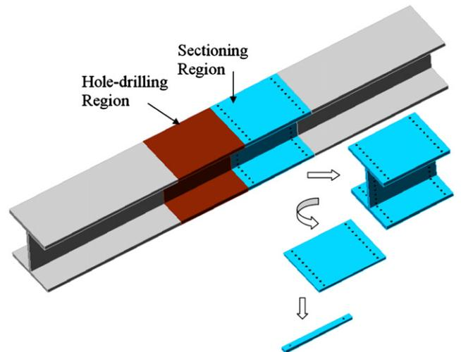
**Fig. 3.** Measurement regions for the sectioning method and the hole-drilling method.
