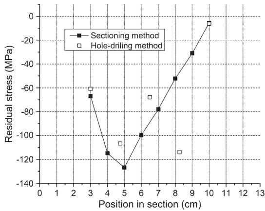
Fig. 11. Comparison of the hole-drilling method and the sectioning method for the R-H-3 web.
