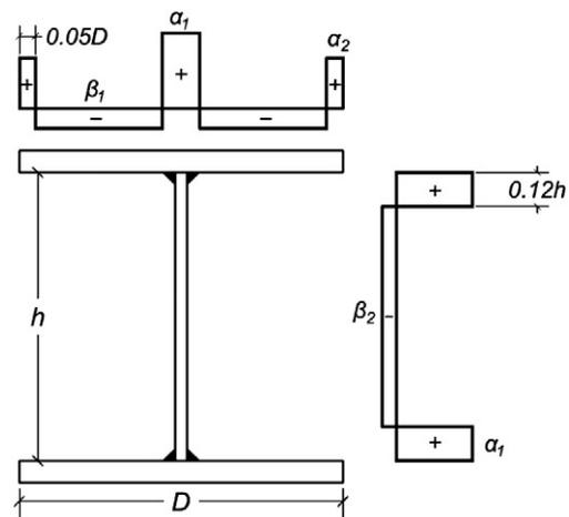
Fig. 12. Simplified residual stress pattern.
