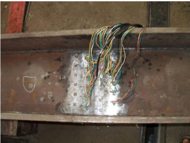
Fig. 5. Test setup of the hole-drilling method.
