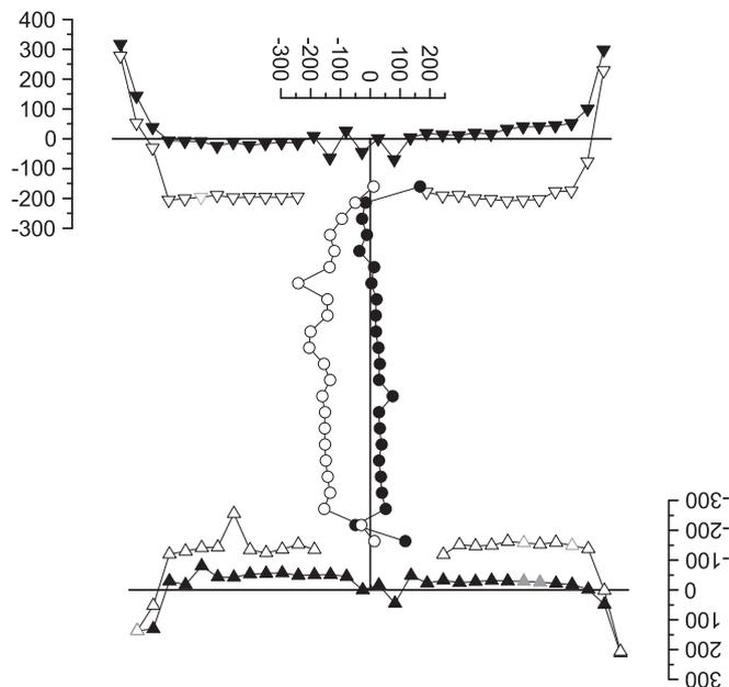
Fig. 8. Residual stress distribution in R-H-7 by sectioning method.
