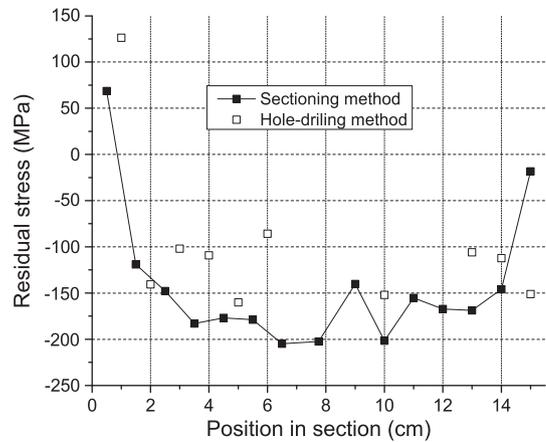
Fig. 9. Comparison of the hole-drilling method and the sectioning method for the R-H-3 top flange.
