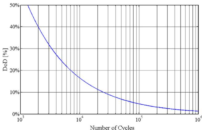
Fig. 1. Wöhler curve for lithium-ion battery.
