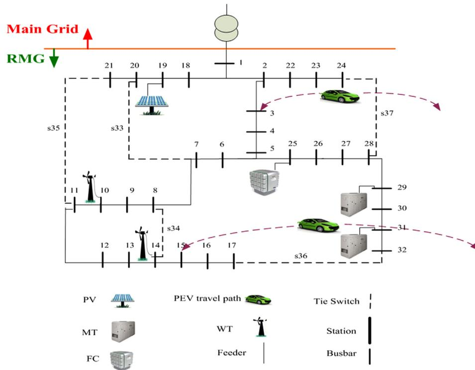
Fig. 3. Schematic of the RMG with DERs and PEV fleet.
