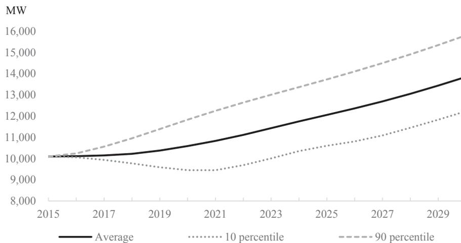
Fig. 6. Sensitivity of installed capacity in the hybrid planning (H) approach to desired transmission capacity. Results shown for average, 10 and 90 percentiles.
