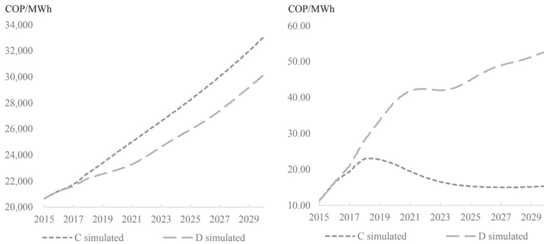
Fig. 4. Simulated (a) usage charges, and (b) compensation charges for centralized (C) and decentralized (D) transmission expansion.
