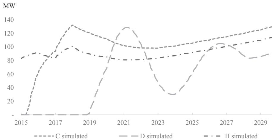
Fig. 5. Simulated annual capacity expansions for centralized (C), decentralized (D) and hybrid (H) approaches.
