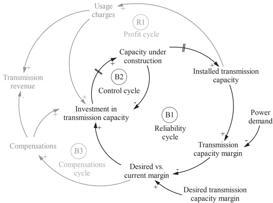
Fig. 1. Causal loop diagram for transmission capacity expansion. Centralized expansion is shown by cycles B1 and B2 in solid lines. Decentralized expansion adds cycles R1 and B3.
