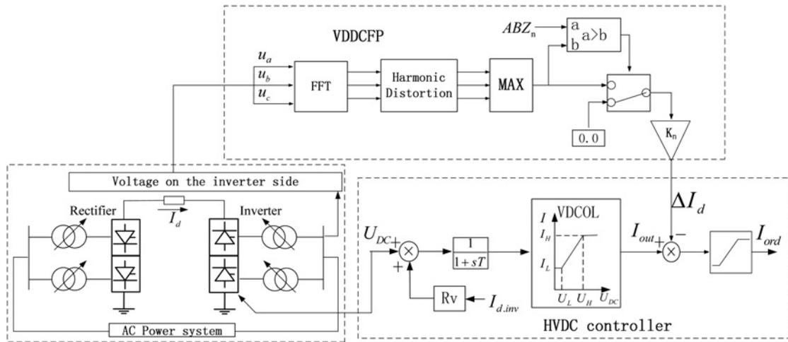
Fig. 5 Detailed block diagram for VDDCFP
