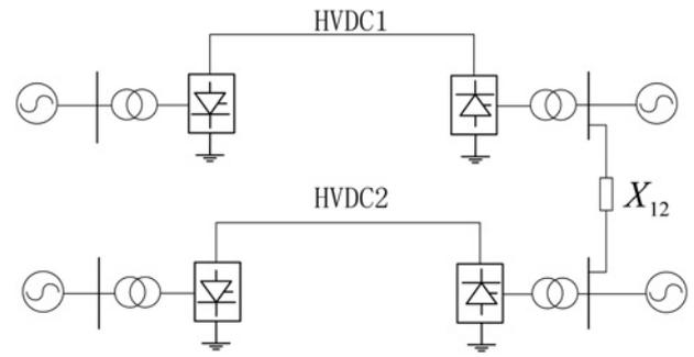
**Fig. 11** Schematic diagram of the typical dual-infeed HVDC test system
