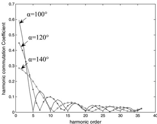
Fig. 4 Relationship between harmonic commutation coefficient and harmonic order
