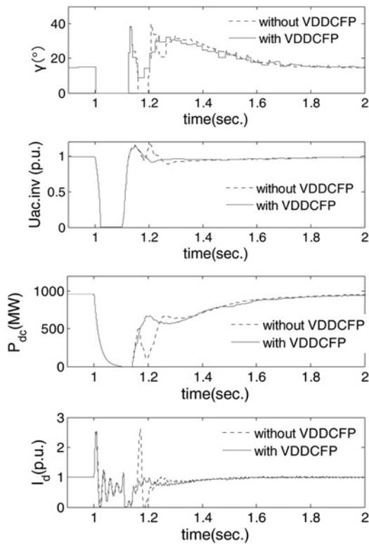
**Fig. 7** System response under three-phase fault ( $\gamma$  is the extinction angle on the inverter side.  $U_{ac,inv}$  is RMS voltage of AC system on the inverter side.  $P_{dc}$  is the HVDC power transmitted to the AC system.  $I_d$  is the Direct current)
