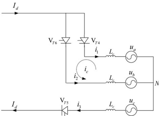
Fig. 2 Equivalent circuit of commutation process
