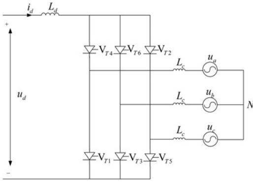
Fig. 1 Equivalent circuit of three-phase full-wave bridge converter
