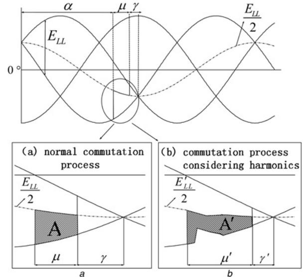
Fig. 3 Harmonic effect on the commutation process
