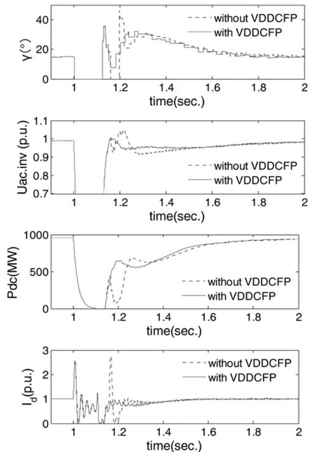
**Fig. 12** Inverter station I responses under single-phase fault in an AC system on the inverter I side ( $\gamma$  is the extinction angle on the inverter side.  $U_{ac,inv}$  is RMS voltage of AC system on the inverter side.  $P_{dc}$  is the HVDC power transmitted to the AC system.  $I_d$  is the direct current)
