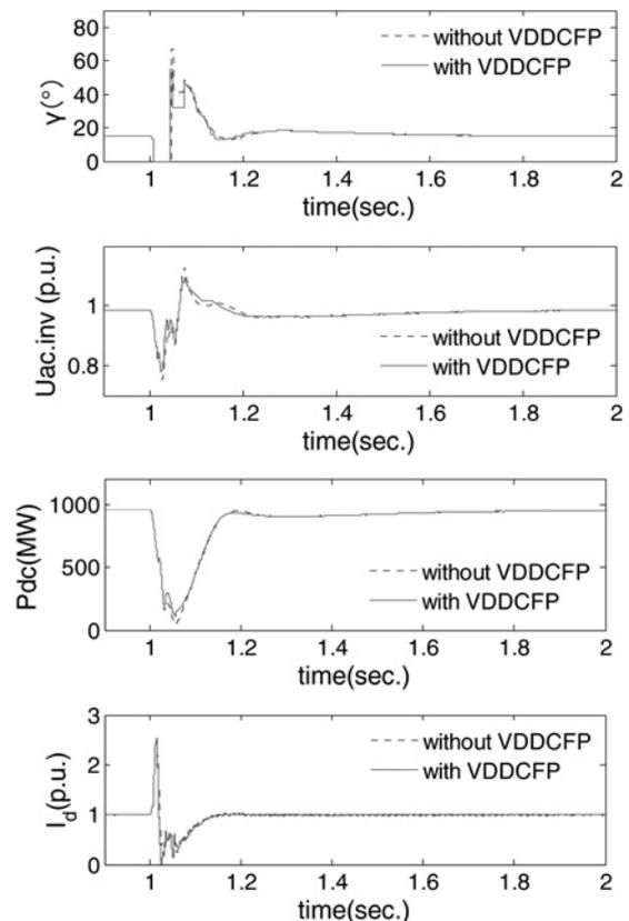
**Fig. 9** System response under single-phase fault ( $\gamma$  is the extinction angle on the inverter side.  $U_{ac,inv}$  is RMS voltage of AC system on the inverter side.  $P_{dc}$  is the HVDC power transmitted to the AC system.  $I_d$  is the direct current)
