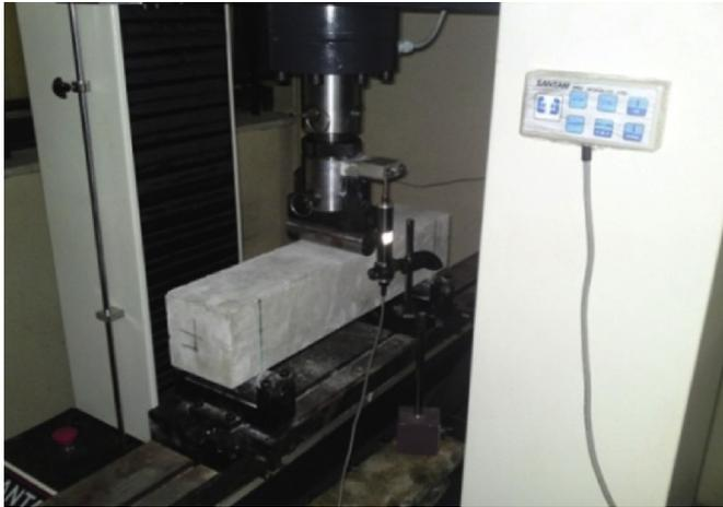
Fig. 4. Flexural strength test using “Universal Machine”.
