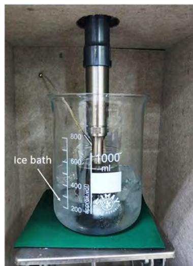
Fig. 1. Ultrasonication of nanofluid.
