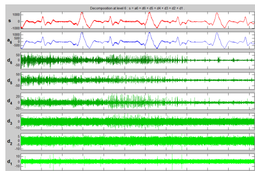
Fig. 11. Feature extraction using db4 wavelet at level 6 for ECG waveform of a patient with Asystole.
