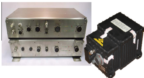
Fig. 3. Longwall shearer localisation measurement solution consisting of an embedded system processor and communications unit (left), and instrumentation grade inertial navigation system (right).
