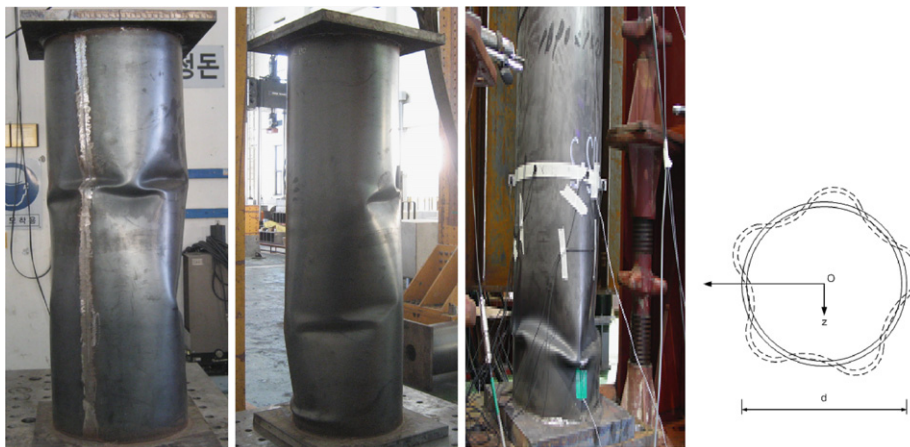
Fig. 2. Failure modes of CHS columns.
