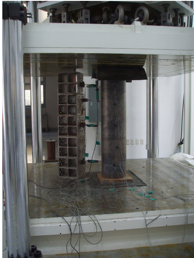
Fig. 4. Test set-up (5000 kN testing machine).
