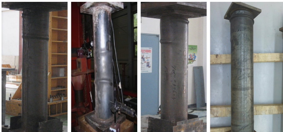
Fig. 5. Collapse modes of circular CFT columns.
