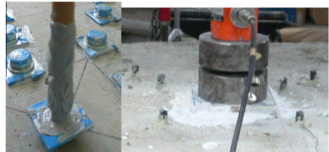
Fig. 8. Screw and nut versus FRP rods setup in slabs.
