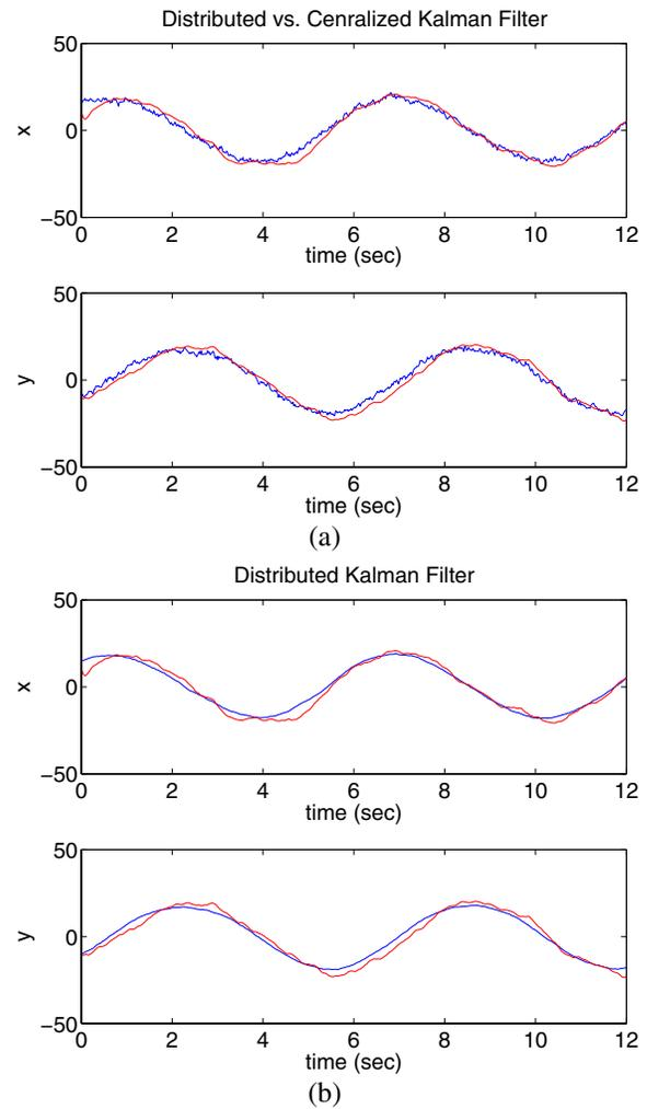
Fig. 4. Distributed position estimation for a moving object by node  $i = 25$ : (a) DKF vs. KF (DKF is the smooth curve in red) and (b) Distributed Kalman filter estimate (in red) vs. the actual position of the object (in blue).
