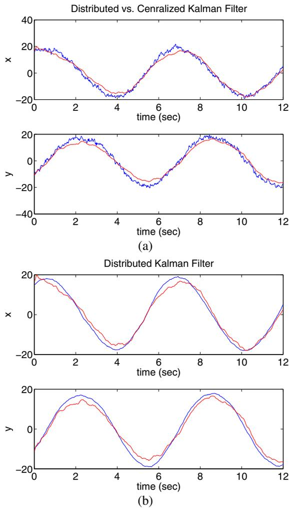
Fig. 3. Distributed position estimation for a moving object by node  $i = 100$ : (a) DKF vs. KF (DKF is the smooth curve in red) and (b) Distributed Kalman filter estimate (in red) vs. the actual position of the object (in blue).
