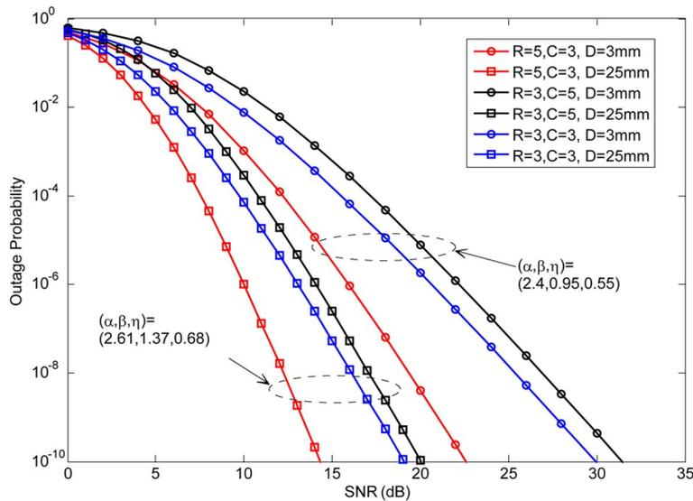
Fig. 7. Outage probability versus SNR for multi-hop parallel FSO system under moderate condition with different  $R$  and  $C$ .
