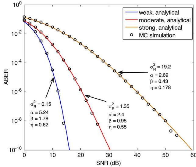
Fig. 2. ABER performance of the multi-hop parallel FSO system with  $R = 3$ ,  $C = 3$  under weak ( $\sigma_R^2 = 0.15$ ), moderate ( $\sigma_R^2 = 1.35$ ), and strong ( $\sigma_R^2 = 19.2$ ) turbulence conditions.
