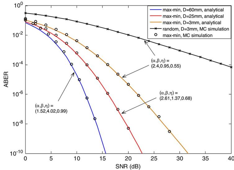
Fig. 3. ABER performance of multi-hop parallel FSO system with  $R = 3$ ,  $C = 3$  under moderate turbulence condition ( $\sigma_R^2 = 1.35$ ) of three different apertures.
