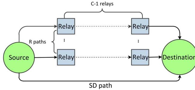
Fig. 1. Structure of multi-hop parallel FSO cooperative communication system.
