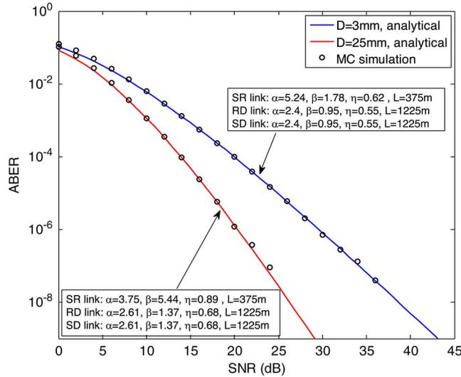
Fig. 10. ABER performance of multi-hop parallel FSO system with non-i.i.d. links over EW fading channels. The structure parameters  $R$  and  $C$  are 1 and 2, respectively.
