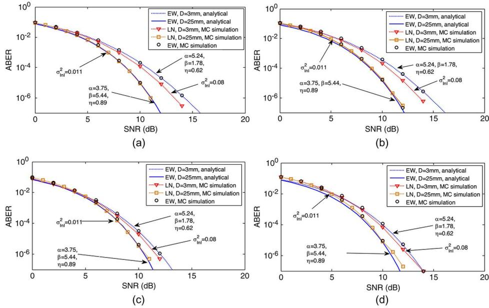
Fig. 9. ABER performance comparison of LN fading channels with that of EW fading channels under weak turbulence condition. The structure of (a) is  $R = 1, C = 2$ . The structure of (b) is  $R = 1, C = 4$ . The structure of (c) is  $R = 3, C = 2$ . The structure of (d) is  $R = 3, C = 4$ .
