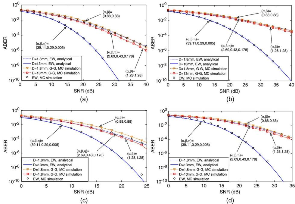
Fig. 8. ABER performance comparison of G-G fading channels with that of EW fading channels under strong turbulence condition. The structure of (a) is  $R = 3$ ,  $C = 3$ . The structure of (b) is  $R = 1$ ,  $C = 3$ . The structure of (c) is  $R = 8$ ,  $C = 3$ . The structure of (d) is  $R = 3$ ,  $C = 6$ .
