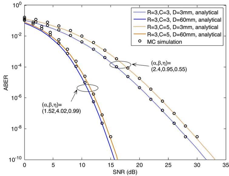
Fig. 5. ABER performance of multi-hop parallel FSO system with different hops in each path under moderate turbulence condition ( $\sigma_R^2 = 1.35$ ).
