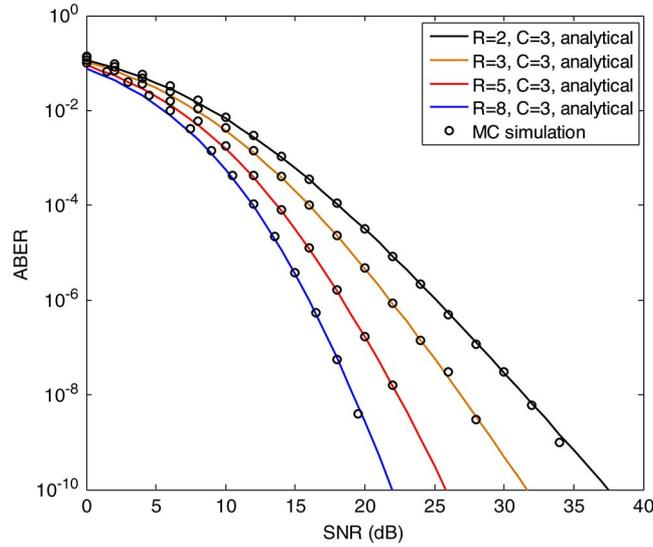
Fig. 4. ABER performance of multi-hop parallel FSO system with different numbers of cooperative path under moderate turbulence condition ( $\sigma_R^2 = 1.35$ ). Link distance  $L = 1225$  m, aperture size  $D = 3$  mm, coherence radius  $\rho_0 = 9.27$  mm, and  $(\alpha, \beta, \eta) = (2.4, 0.95, 0.55)$ .
