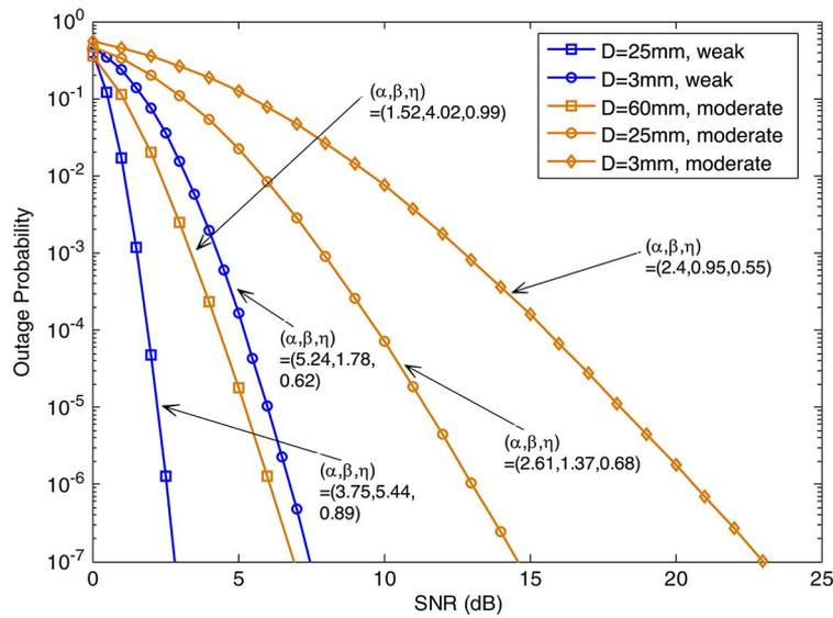
Fig. 6. Outage probability versus SNR for multi-hop parallel FSO system under weak and moderate conditions with  $R = 3$ ,  $C = 3$ .
