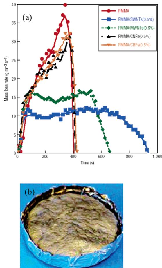
**Figure 11.** (a) Effect of various nanofillers on mass loss rate when PMMA composites are subjected to an external radiant flux of 50 kW m<sup>-2</sup> in nitrogen. (b) Residue from the 0.5 wt % SWNT/PMMA composite after the gasification test showing a free-standing nanotube structure. Reprinted with permission from ref 111.
