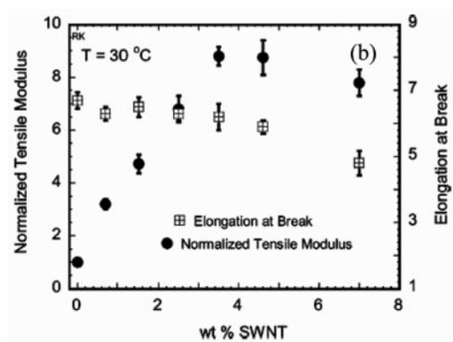
**Figure 6.** (a) Structure of the functionalized SWNT used for the fabrication of PDMS nanocomposite (SWNT not drawn to scale). (b) Composition dependence of the normalized tensile modulus ( $E_{\text{composite}}/E_{\text{PDMS}}$ ) and the elongation at break ( $L_{\text{break}}/L_{\text{initial}}$ ) for SWNT/PDMS nanocomposites. From ref 17.
