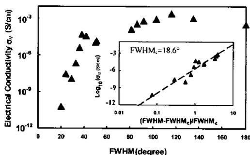
**Figure 8.** Electrical conductivity of a 2 wt % SWNT/PMMA composite along the alignment direction with increasing nanotube isotropy. Nanotube alignment is assessed using X-ray scattering where  $\text{fwhm} = 0$  is perfectly aligned and  $\text{fwhm} = 180$  is isotropic. Inset: a log–log plot of electrical conductivity vs reduced fwhm determines the critical alignment,  $\text{fwhm}_c$ . Reprinted with permission from ref 23. Copyright 2005 American Physical Society.
