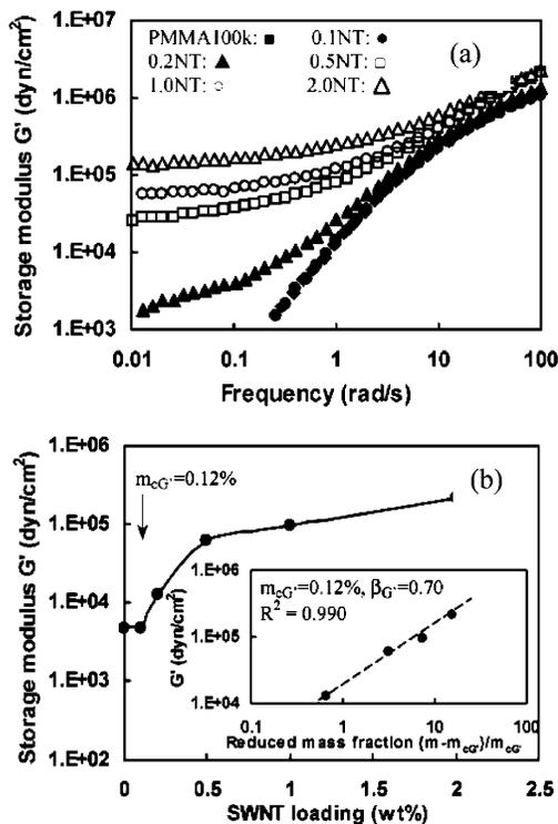
**Figure 9.** (a) Storage modulus ( $G'$ ) vs shear frequency for SWNT/PMMA nanocomposites with various nanotube loadings from 0 to 2.0 wt %. (b)  $G'$  as a function of the nanotube loading for SWNT/PMMA nanocomposites at a fixed frequency, 0.5 rad/s. Inset: a power law plot of  $G'$  vs reduced mass fraction on a logarithmic scale. From ref 37.
