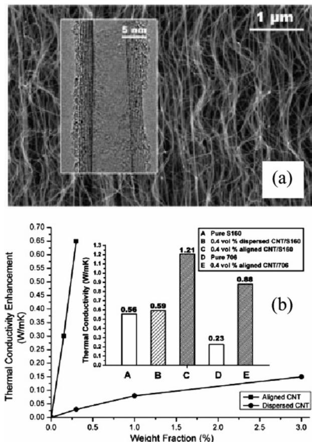
**Figure 10.** (a) SEM image of the side view of an aligned MWNT array. Inset: a high-resolution TEM image of an isolated MWNT showing eight nested nanotubes. (b) Thermal conductivity enhancement ( $\kappa_{\text{composite}} - \kappa_{\text{matrix}}$ ) vs weight fraction of MWNT in both aligned and unaligned nanocomposites. Inset: thermal conductivity for selected MWNT/silicone elastomer composites. Reprinted with permission from ref 64. Copyright 2005 Wiley-VCH.
