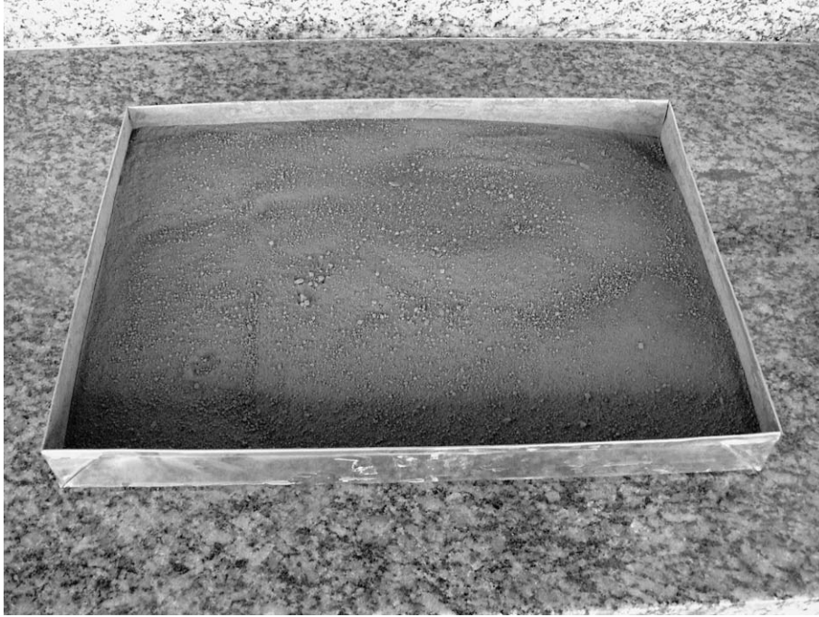
Fig. 5. Sludge oven-dried for 24 h at 110 °C.
