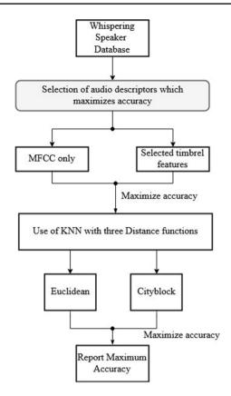
Fig. 1 Speaker identification system block diagram
