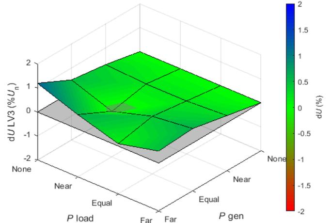
Figure 5. Difference of relative voltage changes at node LV3 between  $Q_{GEN} = 0$  and  $Q_{GEN} = f(P_{GEN}, U)$  reactive power regulation regarding the desired voltage in LV network with cable lines
