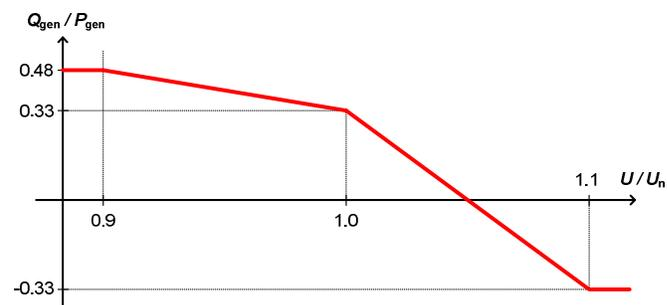
Figure 1. Proposed optimized reactive power characteristic  $Q_{GEN} = f(P_{GEN}, U)$  of DGs in the LV network
