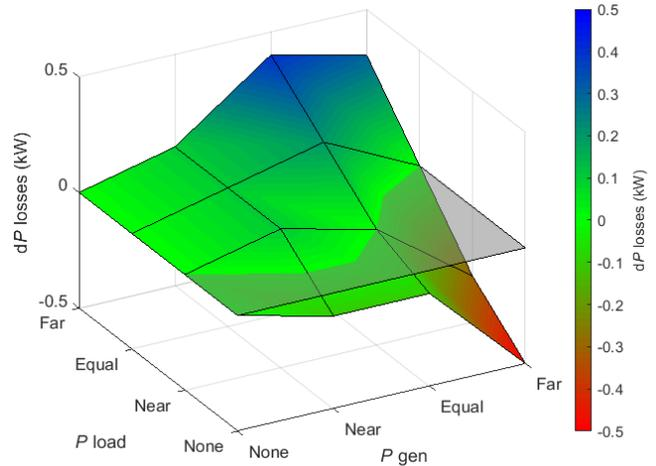
Figure 7. Difference of cumulative losses on the MV/LV transformer and LV network between  $Q_{GEN} = 0$  and  $Q_{GEN} = f(P_{GEN}, U)$  reactive power regulation in LV network with cable lines
