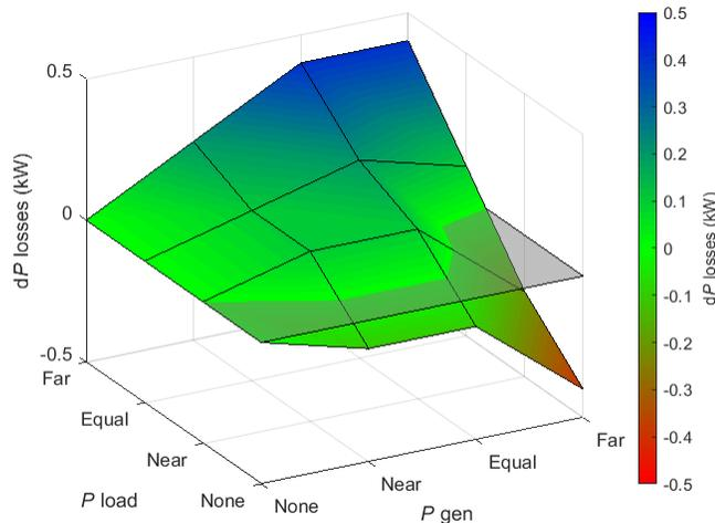
Figure 6. Difference of cumulative losses on the MV/LV transformer and LV network between  $Q_{GEN} = 0$  and  $Q_{GEN} = f(P_{GEN}, U)$  reactive power regulation in LV network with overhead lines
