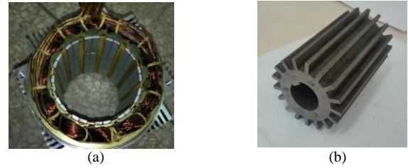
Fig. 11. 12-slot/17-pole FRPMM prototype: (a) Stator; (b) Rotor.
