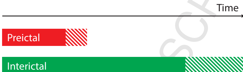
Figure 4: Practice to prevent the convolutional neural network from overfitting the data during training. Twenty-five percent of later samples (diagonal lines) from preictal and interictal recordings in the training dataset are used for monitoring and the rest are used for training.
