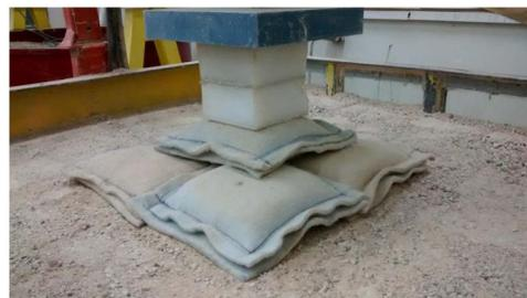
Fig. 22. The typical arrangement of the improvement using 5 geobags.
