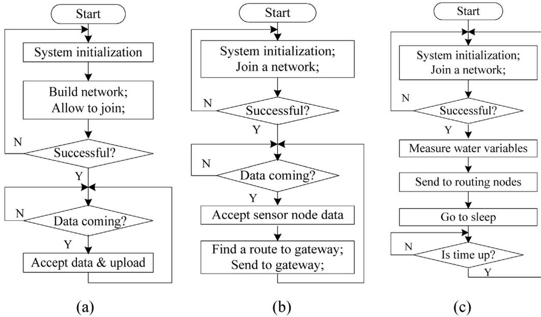
Fig. 6 – Software flow for WSN nodes: (a) gateway node; (b) routing node; (c) sensor node.
