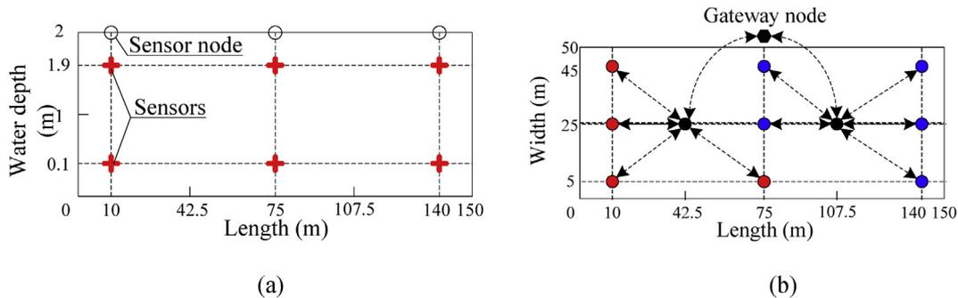
Fig. 10 – Measurement experiments: (a) deployment of sensors; (b) WSN topology.
