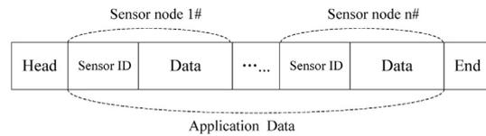
Fig. 8 – Structure of compound data frame.
