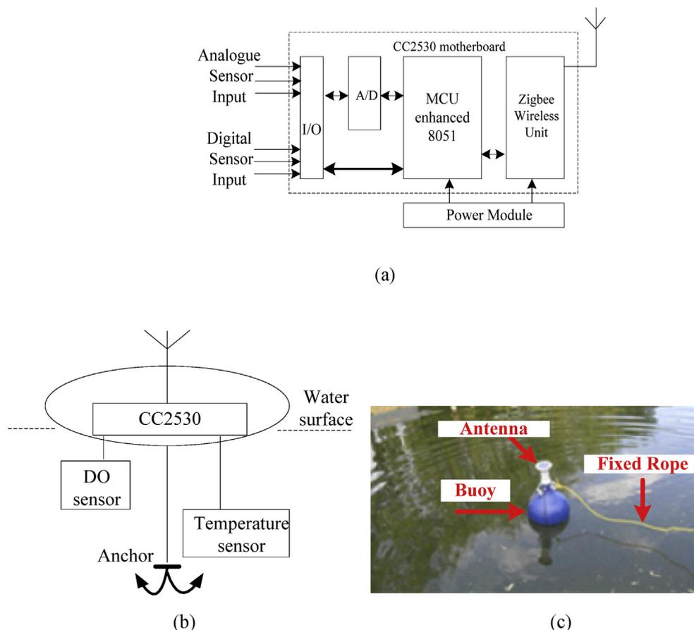
Fig. 4 – Sensor node: (a) schematic diagram; (b) appearance diagram; (c) physical appearance.
