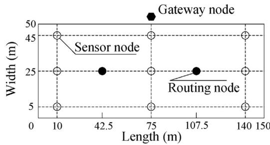
Fig. 9 – Deployment of WSN nodes.
