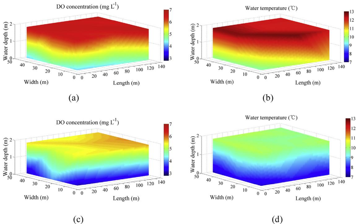
**Fig. 11 – Three-dimensional distributions of measurements: (a) DO concentration at 11:00; (b) water temperature at 11:00; (c) DO concentration at 23:00; (d) water temperature at 23:00.**
