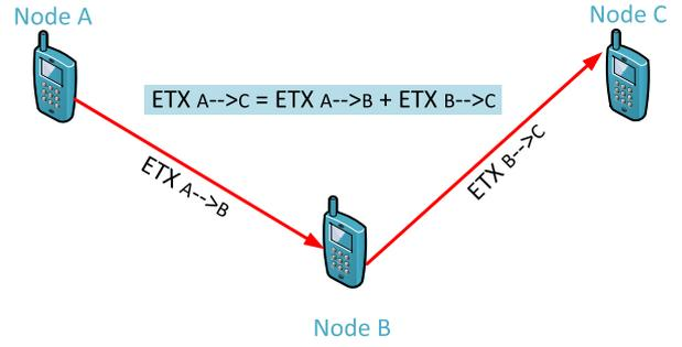
Fig. 2. Two hop neighbor set - ETX calculation for routing table computation.
