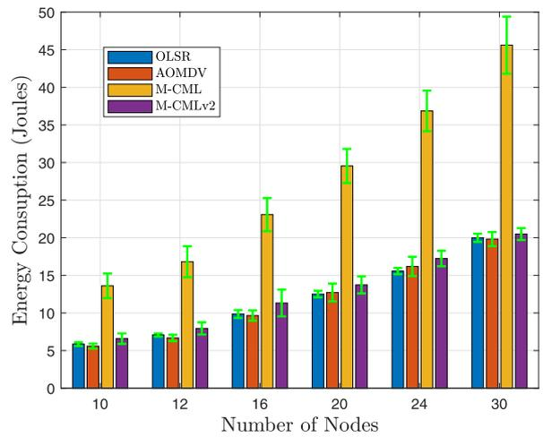
Fig. 11. Measurement of total energy consumption vs. various node densities.
