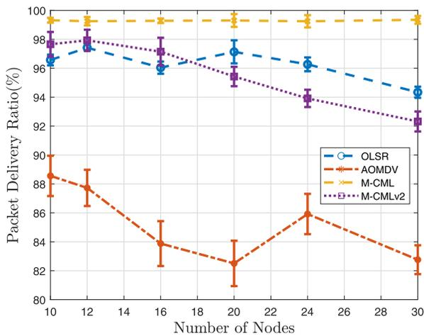
Fig. 5. Measurement of packet delivery ratio vs. various node densities.
