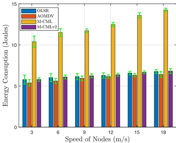
Fig. 10. Measurement of total energy consumption vs. various speeds of nodes.
