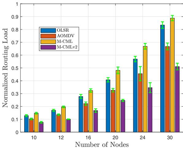
Fig. 9. Measurement of normalized routing load vs. various node densities.
