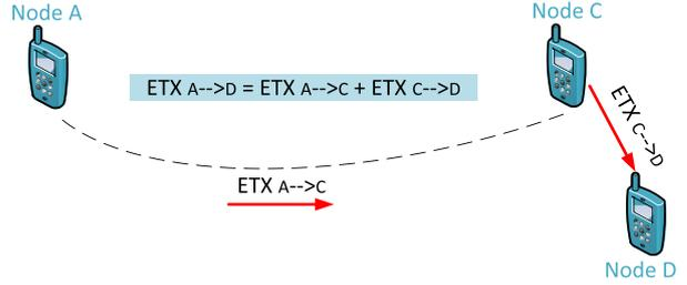
Fig. 3. Topology set - ETX calculation for routing table computation.
