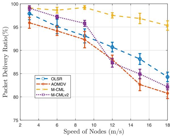
Fig. 4. Measurement of packet delivery ratio vs. various speeds of nodes.
