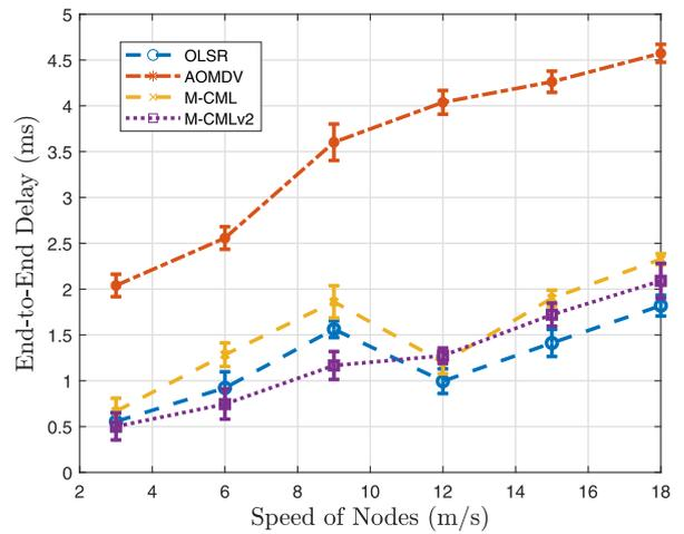
Fig. 6. Measurement end-to-end delay vs. various speeds of nodes.
