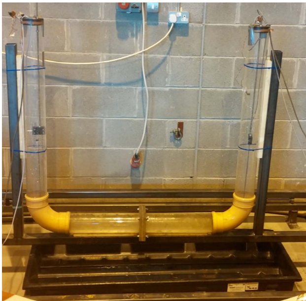
Fig. 3. Tuned Liquid Column Damper used in the experimental analysis.
