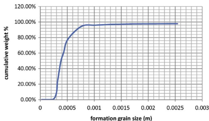
Fig. 2. Formation grain size distribution (adapted from Iranian oil company).
