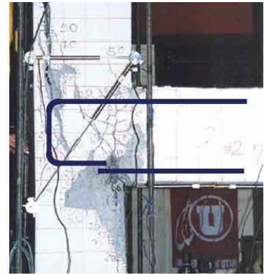
(c) Anchorage failure [Pantelides et al. , 2002]
