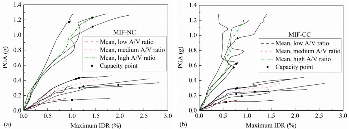
Figure 7. IDA curves for (a) MIF-NC and (b) MIF-CC frames.
