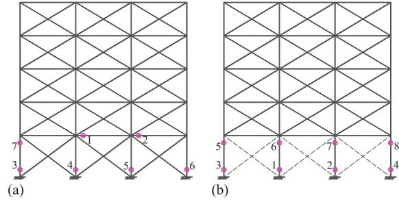
**Figure 9.** Formation of the plastic hinges for: (a) MIF-NC and (b) MIF-CC frames (circular dots indicate beam and column hinges; numbers represent the sequence of occurrence of the plastic hinges; and diagonal dotted lines indicate collapse of infills).
