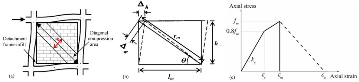
**Figure 5.** (a) Strut model analogy of the infill, (b) deformation, and (c) axial stress–axial strain relationship of the infill compression strut.
