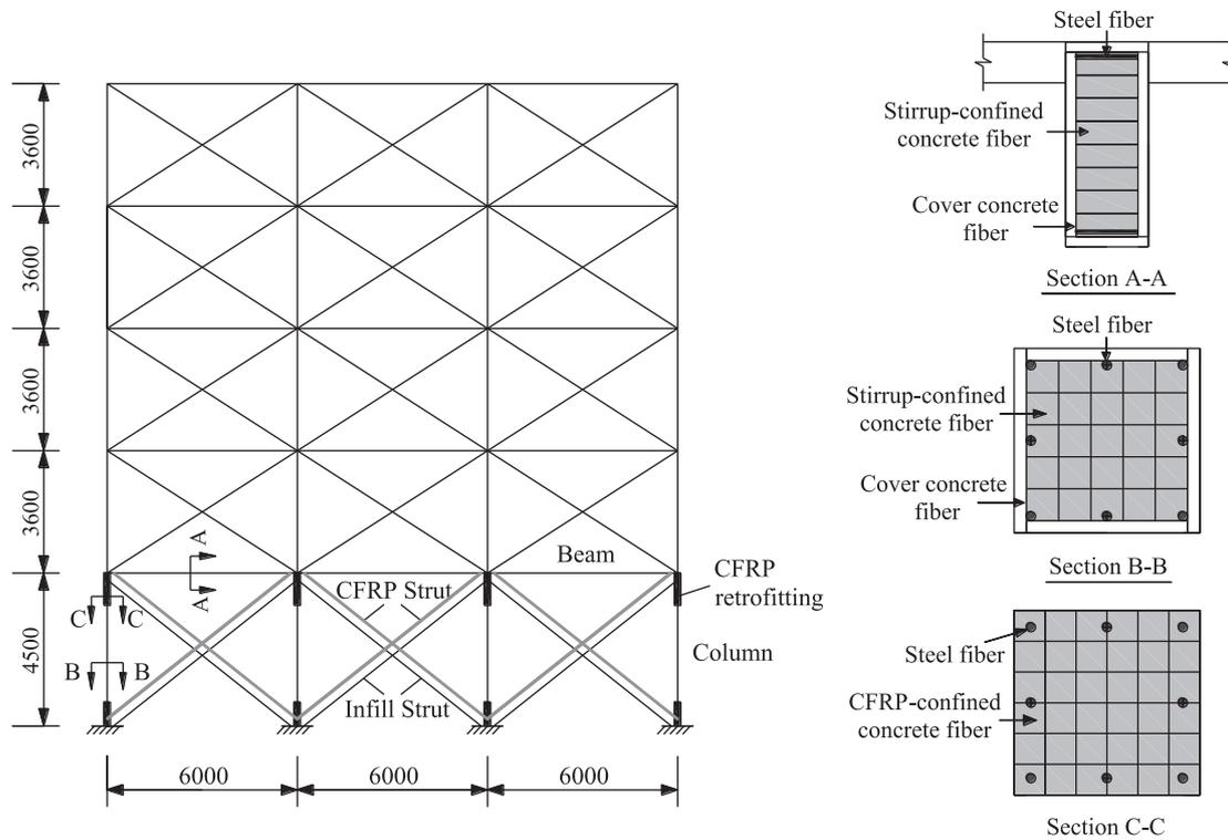
**Figure 3.** Finite element model for retrofitting scheme II (dimensions in mm).
