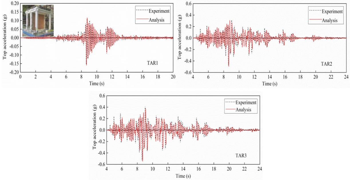
Figure 6. Comparison of top acceleration time histories between the experimental and analytical results.
