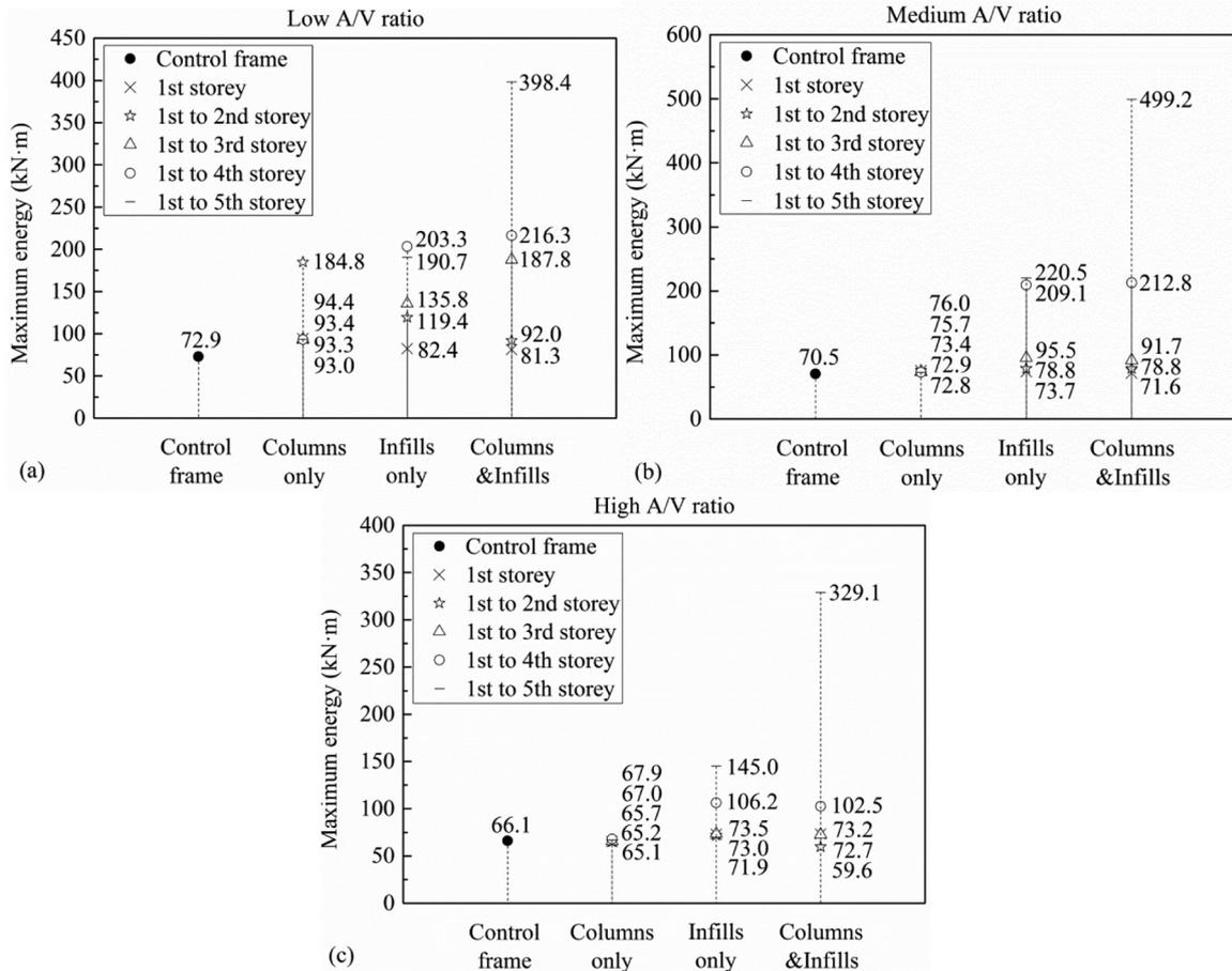
**Figure 14.** Mean maximum energy dissipated by the control and retrofitted frames: (a) low A/V ratio, (b) medium A/V ratio, and (c) high A/V ratio.
