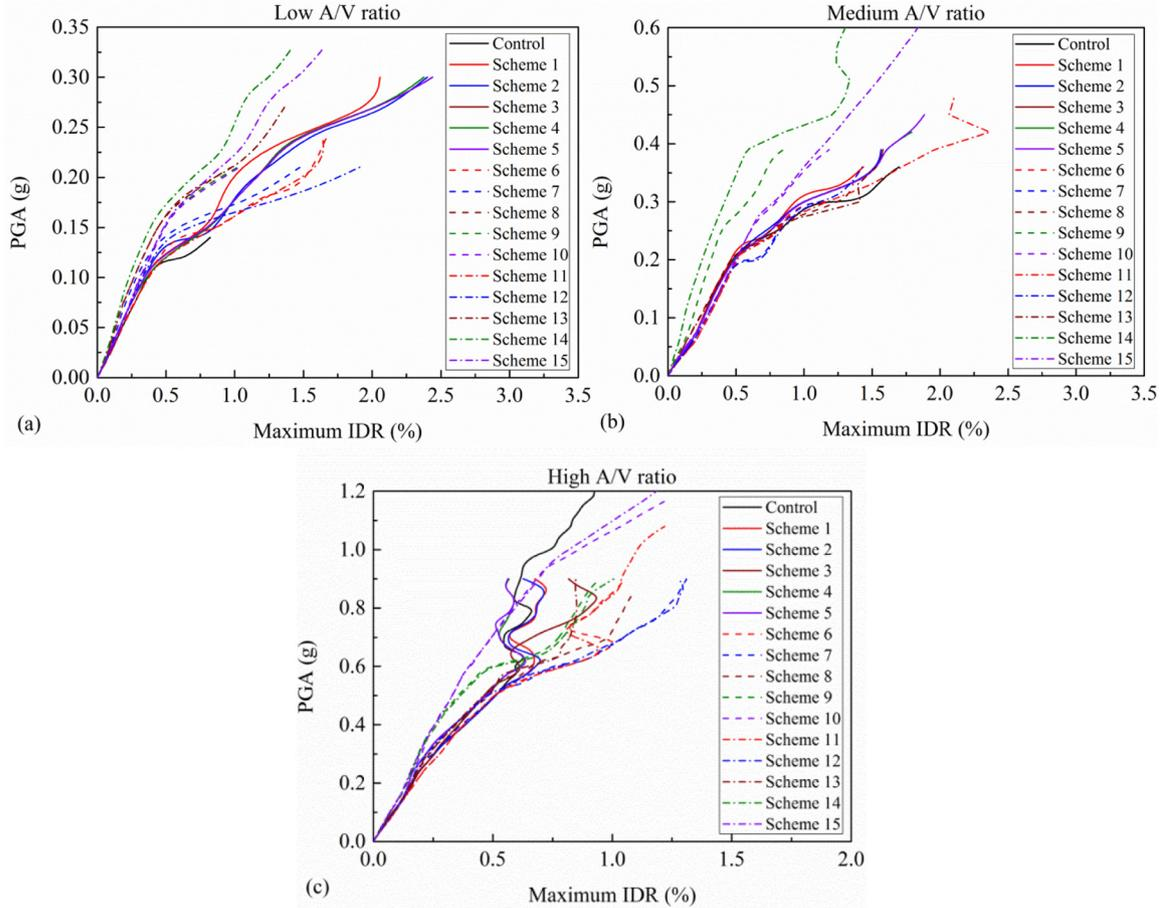
**Figure 10.** Mean IDA curves for the control and retrofitted frames: (a) low A/V ratio, (b) medium A/V ratio, and (c) high A/V ratio.
