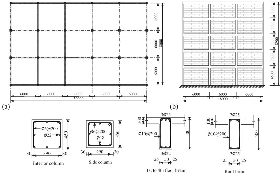
**Figure 1.** (a) Plan and (b) elevation of the studied building (units: mm).
