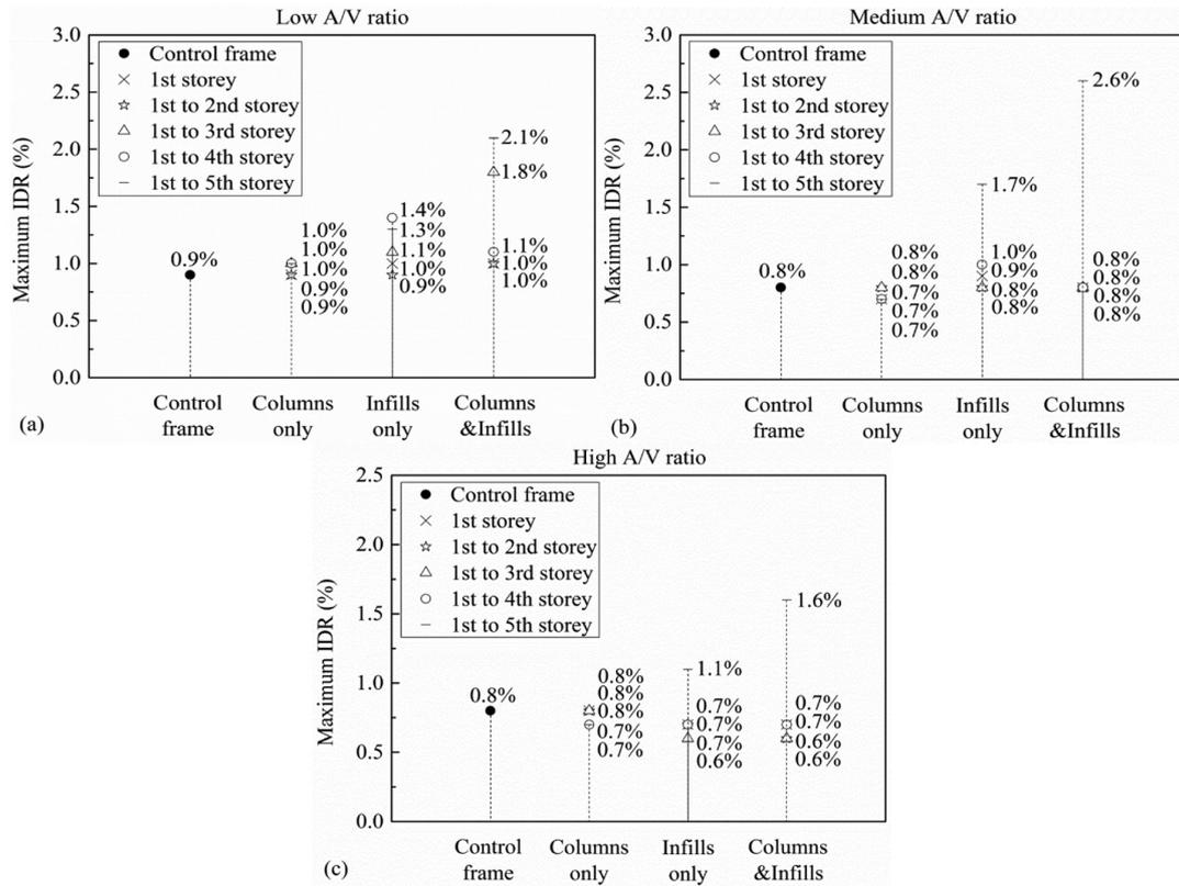
**Figure 13.** Mean maximum IDR capacity for the control and retrofitted frames: (a) low A/V ratio, (b) medium A/V ratio, and (c) high A/V ratio.
