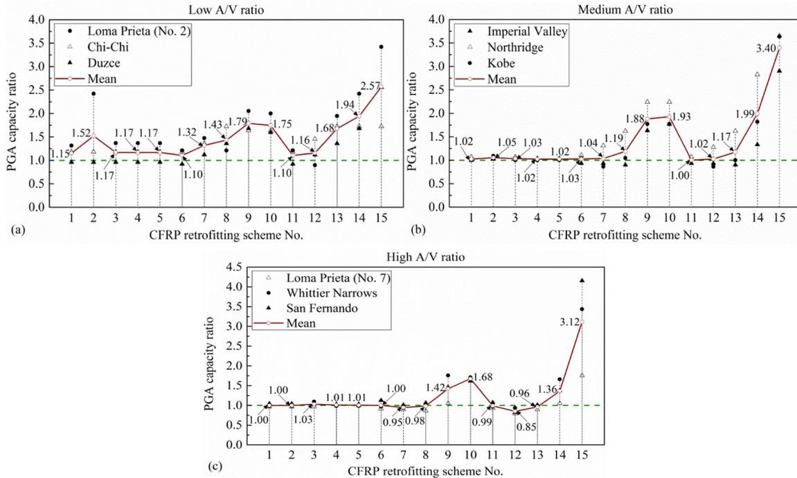
**Figure 11.** PGA capacity ratio of retrofitted frames: (a) low A/V ratio, (b) medium A/V ratio, and (c) high A/V ratio.
