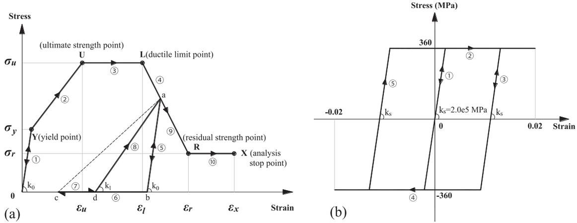
Figure 4. Cyclic stress–strain relationship of: (a) concrete and (b) steel bars.
