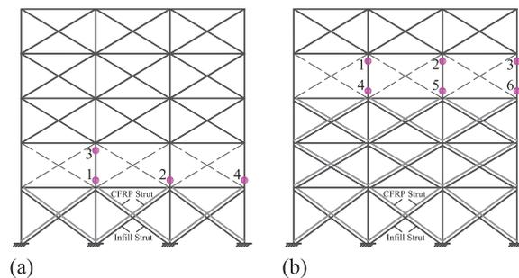
**Figure 12.** Formation of the plastic hinges for retrofitting: (a) scheme 6 and (b) scheme 8.
