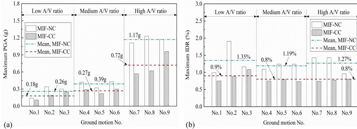
**Figure 8.** (a) Maximum PGA and (b) maximum IDR capacities for MIF-NC and MIF-CC frames.
