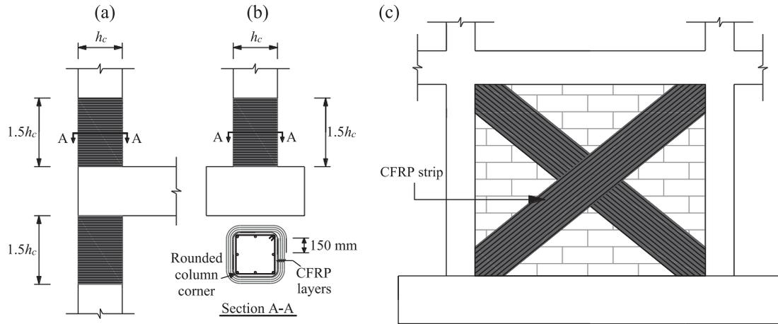
**Figure 2.** CFRP strip configuration used for: (a) column ends, (b) bottom of first story columns, and (c) masonry infills.
