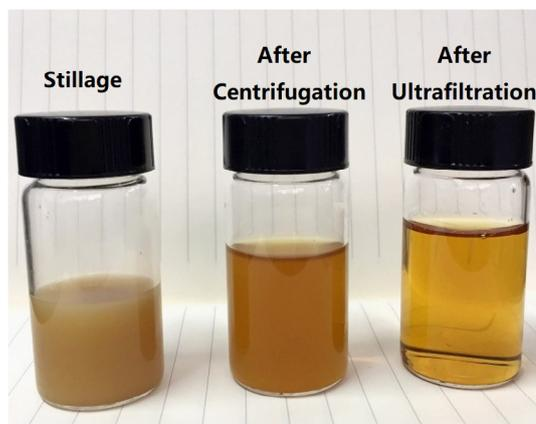
Fig. 2. Comparison of stillage with centrifugation and ultrafiltration treatment.
