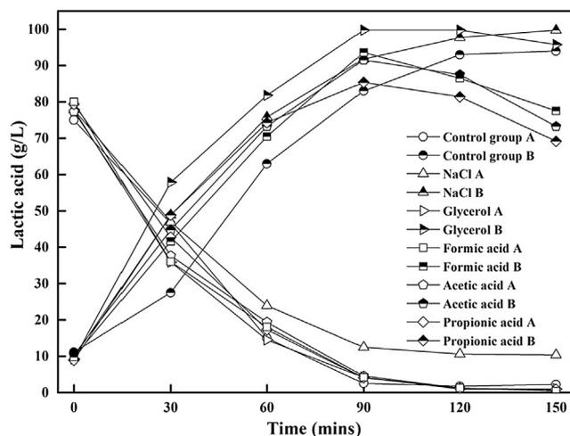
Fig. 4. Change of lactic acid content in electro dialysis process.
