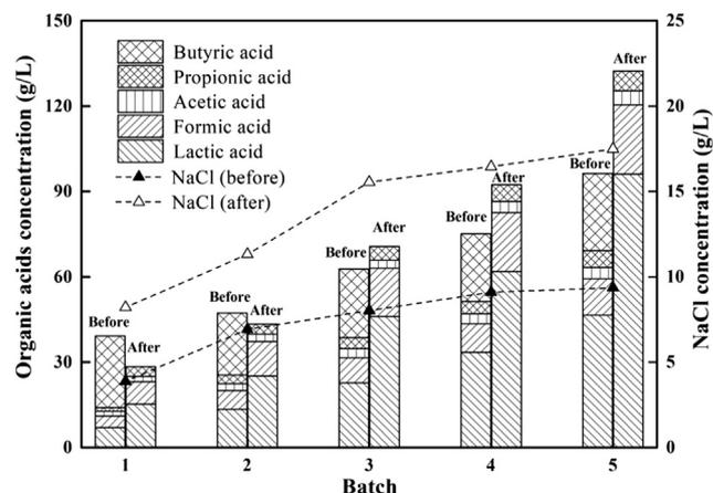
Fig. 3. Content of organic acids and NaCl in stillage before and after distillation.
