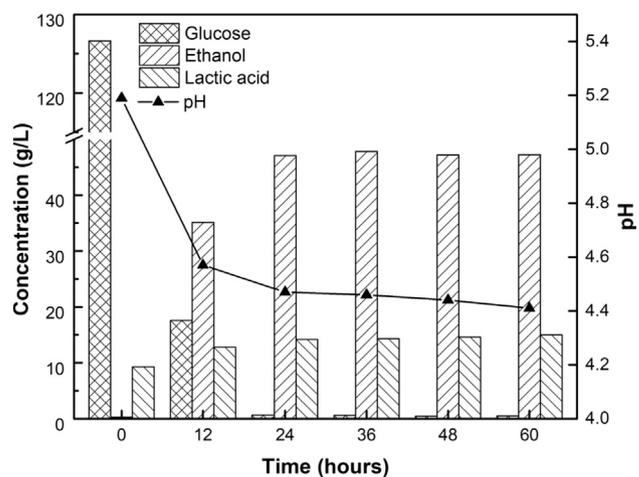
Fig. 7. Change of pH and the concentration of glucose, ethanol and lactic acid.
