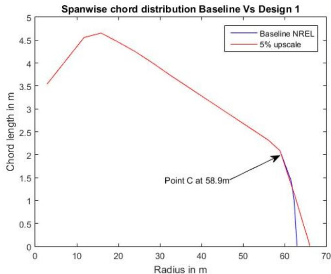
559 Fig. 14 NREL Vs New Blade design chord length distribution
