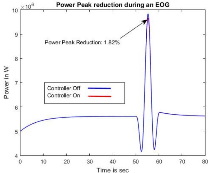
Fig. 22 Wind Turbine Power Peak reduction during an EOG for 10% tip swept rotor.
