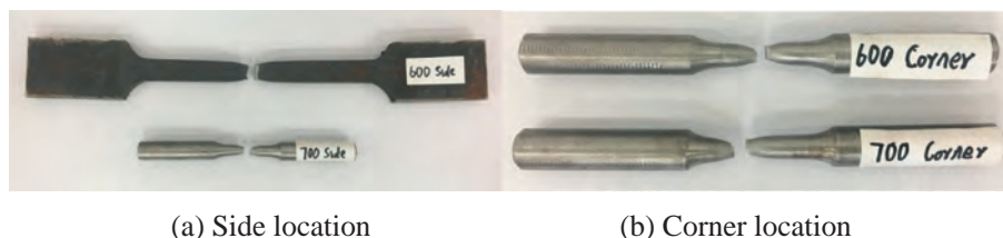
Fig. 10. Fracture morphology of specimens.
