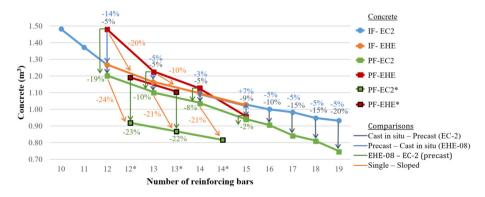
Fig. 5. Quantity of concrete for shallow foundations with different numbers of 12 mm diameter reinforcing bars. Terminology: cast in situ (1); precast (P); rigid (R); flexible (F); calculated with EC-2 (EC2); calculated with EHE-08 (EHE).
