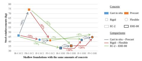
Fig. 3. Quantity of steel reinforcement in shallow foundations with the same amounts of concrete. Terminology: cast in situ (1); precast (P); rigid (R); flexible (F); calculated with EC-2 (EC2); calculated with EHE-08 (EHE).
