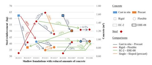
Fig. 4. Diagram of the quantity of concrete and steel reinforcement for shallow foundations with reduced amounts of concrete. Terminology: cast in situ (1); precast (P); rigid (R); flexible (F); calculated with EC-2 (EC2); calculated with EHE-08 (EHE).
