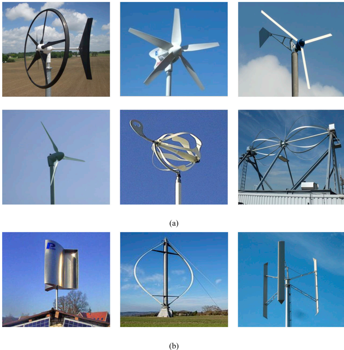
Fig. 4. Examples of common existing (a) Horizontal axis wind turbines (HAWTs) and (b) Vertical axis wind turbines (VAWTs). (Source: different websites; see references). 1 http://www.prweb.com/releases/2010/07/prweb4281554.htm . 2 https://www.energyonthehook.com/Eclectic-Energy-D400-Wind-Generator-p/ecl400.htm . 3 http://www.fortiswindenergy.com/montana/ . 4 http://www.renugen.co.uk/wind-energy-solutions-wes5-tulipo-2-5-kw-wind-turbine/ . 5 http://www.windworks.org/cms/index.php?id=64&tx_ttnews%5Btt_news%5D=95&cHash=702973dca5ecf0c94d5d52e4e6094888 . 6 https://www.alibaba.com/product-detail/WindWall-3kW-Windturbine_109199832.html . 7 http://www.netzeroguide.com/savonius-wind-turbine/ . 8 https://en.wind-turbine-models.com/turbines/93-dormier-darrieus-55 . 9 http://lifefreeenergy.com/v/vertical-wind-turbine.html/page/2/ .
