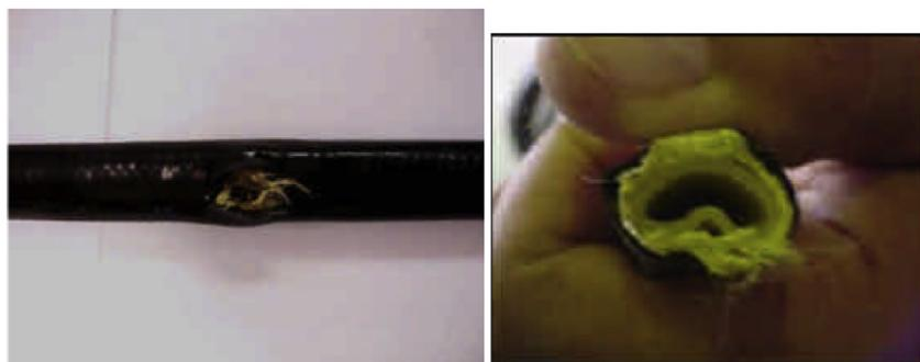
Fig. 11. Hydraulic hose failed in operation (Rabelo, 2013).
