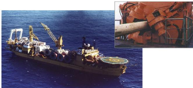
Fig. 8. Pipe laying support vessel (PLSV) and its tensioner (Rabelo, 2013).
