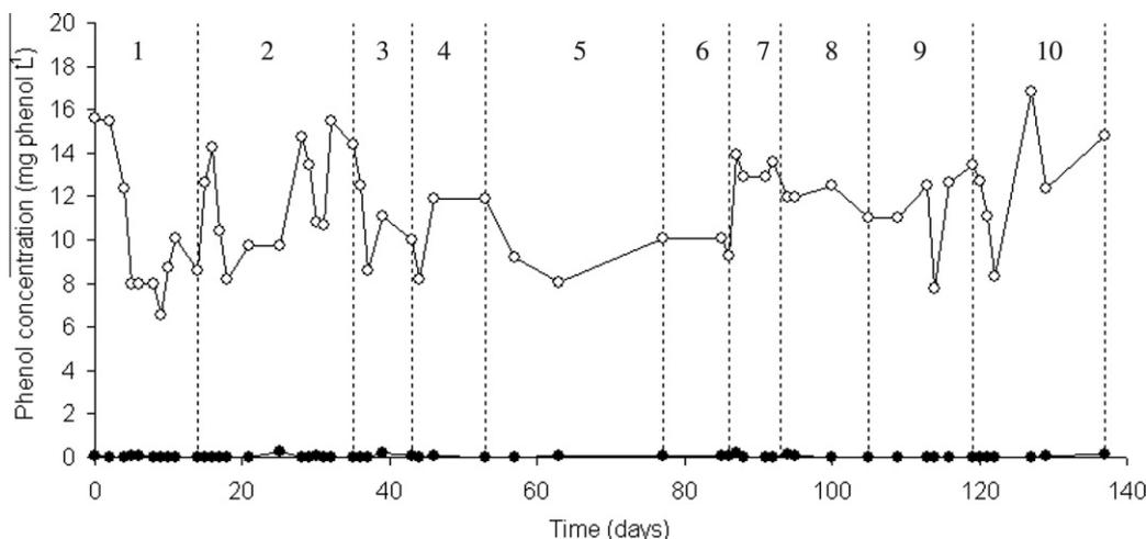
**Fig. 3.** MBR operation for the treatment of industrial wastewater containing phenol (○ influent phenol concentration; ● effluent phenol concentration). (Periods: 1 (HRT = 3.6 days), 2 (HRT = 1.9 days), 3 (HRT = 1.3 days), 4 (HRT = 1.9 days), 5 (HRT = 3.6 days), 6 (HRT = 1.3 days), 7 (HRT = 1.1 days), 8 (HRT = 0.75 days), 9 (HRT = 0.5 days), 10 (HRT = 0.45 days).
