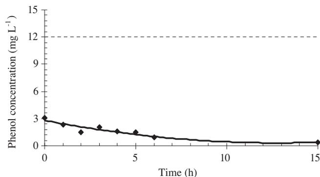
**Fig. 2.** Phenol biological removal rate in the MBR. Phenol concentration in the mixed liquor (■) and phenol concentration in the influent (—).
