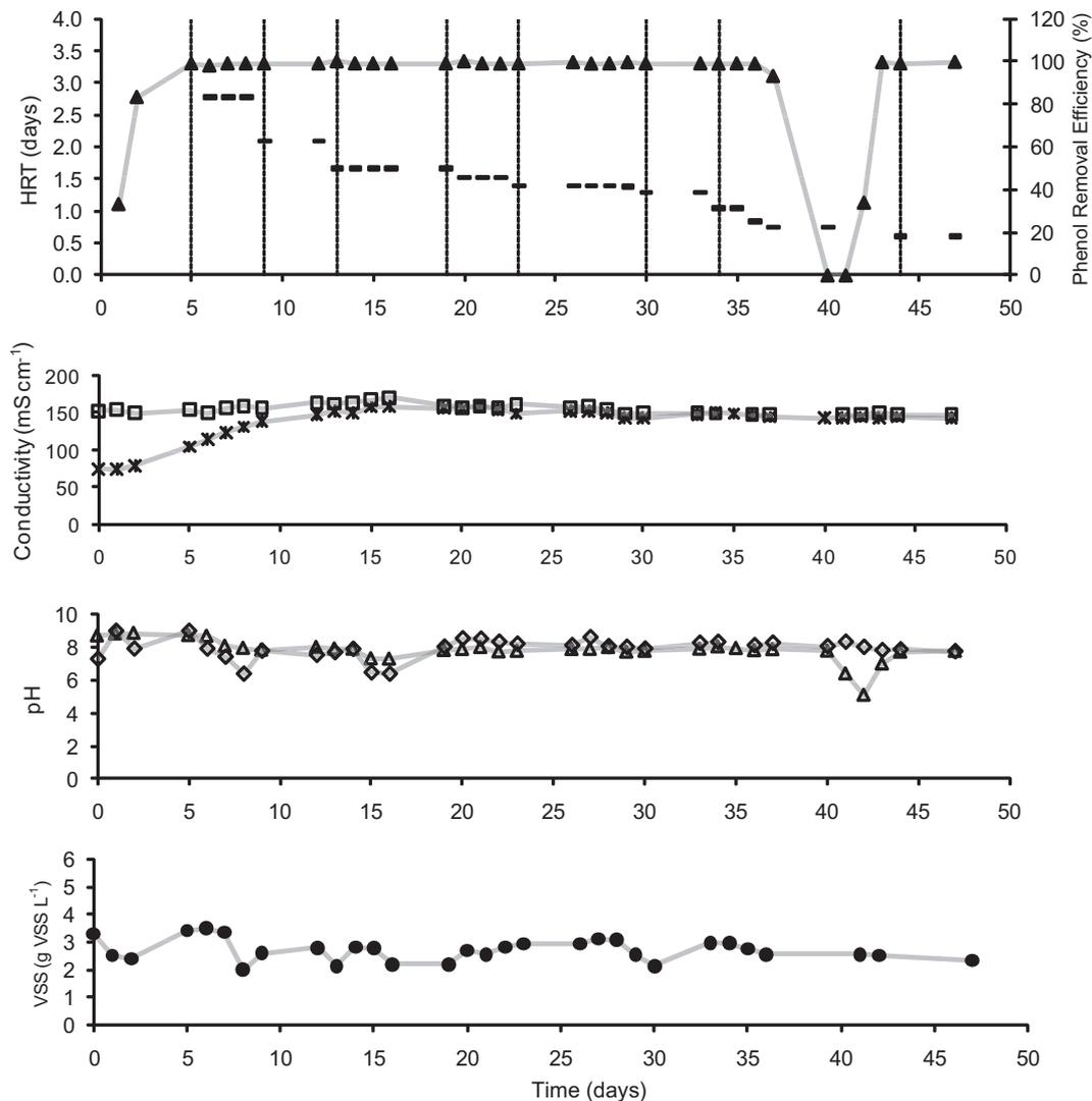
**Fig. 4.** MBR operation for the treatment of industrial wastewater containing phenol at pilot plant conditions (phenol removal efficiency ( $\blacktriangle$ ); HRT ( $\text{—}$ ); influent conductivity ( $\square$ ) effluent conductivity ( $\times$ ); influent pH ( $\diamond$ ) effluent pH ( $\Delta$ ); VSS concentration in the reactor ( $\bullet$ )).
