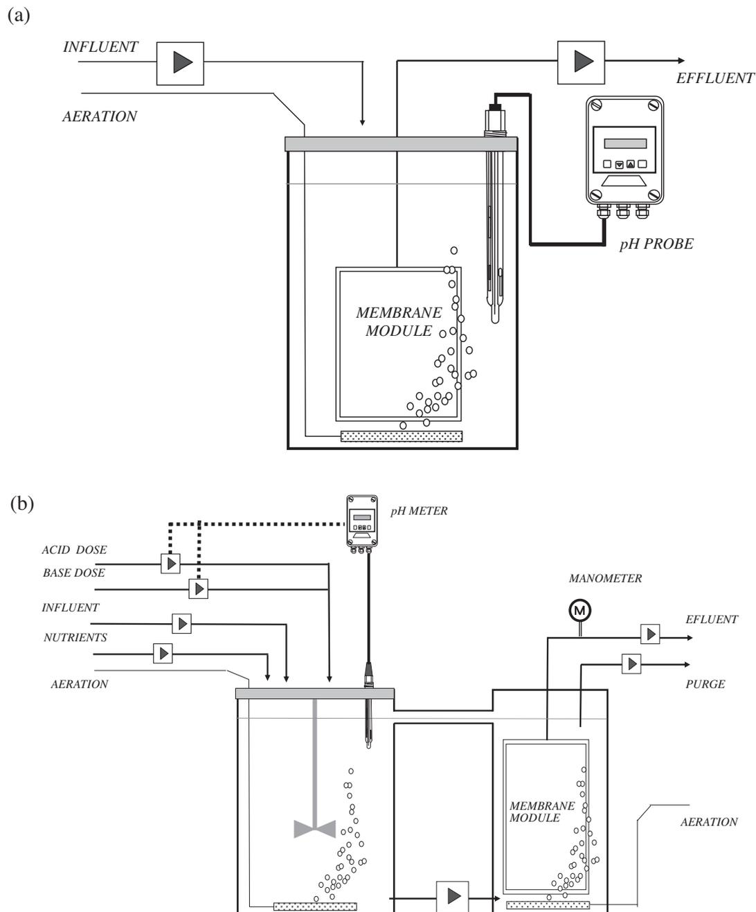
Fig. 1. Scheme of the lab-scale MBR (a) and the pilot plant MBR (b) used in this study.
