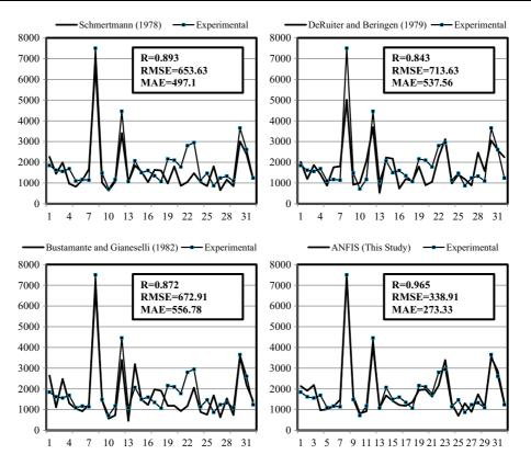
Fig. 4 A comparative plot of experimental and predicted P<sub>u</sub> (kN) values using different models for test data
