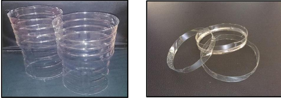
Fig. 1. Ring-shaped PET fibers.
