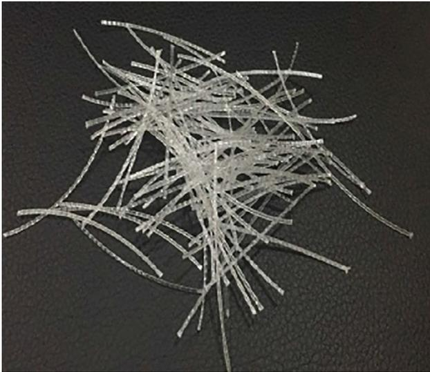
Fig. 5. Manufactured synthetic macro-fibers.
