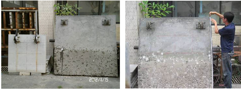
Fig. 15. Appearance of FRC sluice gates after they were removed from their embankments.
