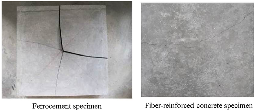
Fig. 10. Concrete specimens produced cracks after the impact test.
