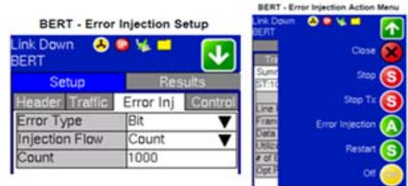
Fig 10. Error injection/activation settings for BERT
