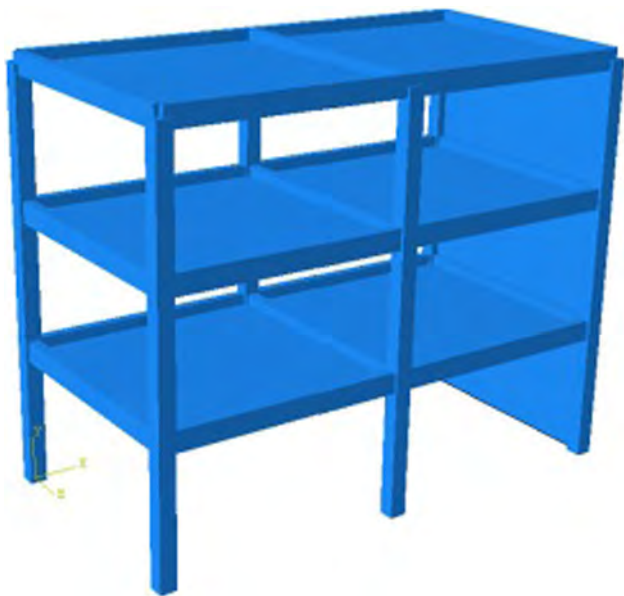
Fig. 16. Three-dimensional FE model of the shaking table specimen.
