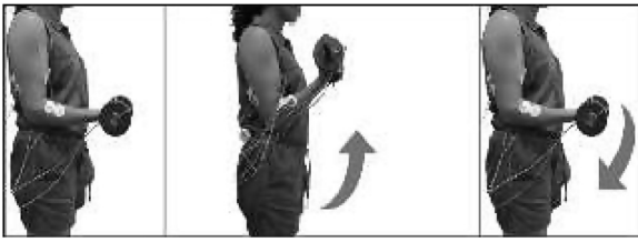
Fig. 13. Arm motion to obtain real biceps EMG signals. The arm of the subject is initially at rest and holding a weight of 4 kg, with the elbow touching the body (left). The subject then lifts the weight with the elbow touching the body (center). Finally, the arm returns to the original resting position (right). This motion is repeated three times.
