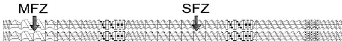
**Scheme 1.** Screw configuration by assembling diverse screw elements (conveying, kneading, mixing and sealing) on screw shafts in a modular design. MFZ: main feeding zone. SFZ: side feeding zone.
