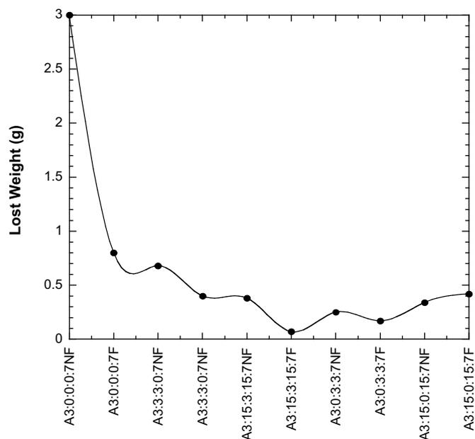
**Fig. 3.** Plot of lost weight in gravel–asphalt adhesion experiment for all samples.
